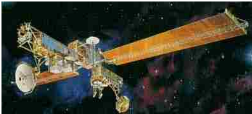
Figure 2. A Milstar communications satellite with two opposing 4.3 kW tensioned photovoltaic blanket winglets each supported by a compression column.
