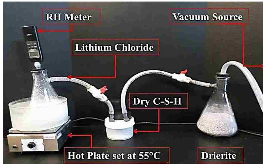
Figure 3.5: 11% Drying System Set-up
