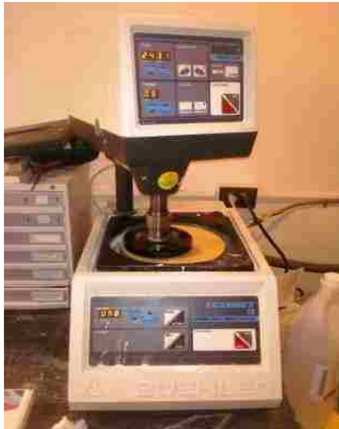
Figure 3.15: Polishing apparatus for preparation on nanoindentation samples
