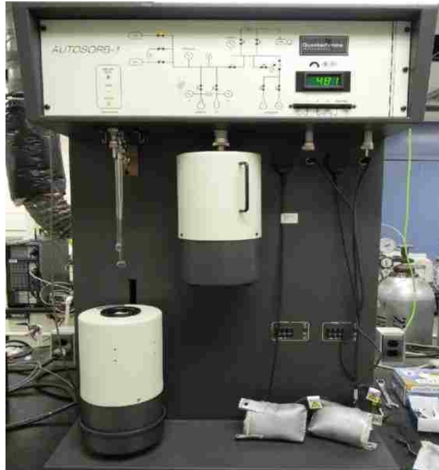
Figure 3.17: 3.23 BET N2 testing system
