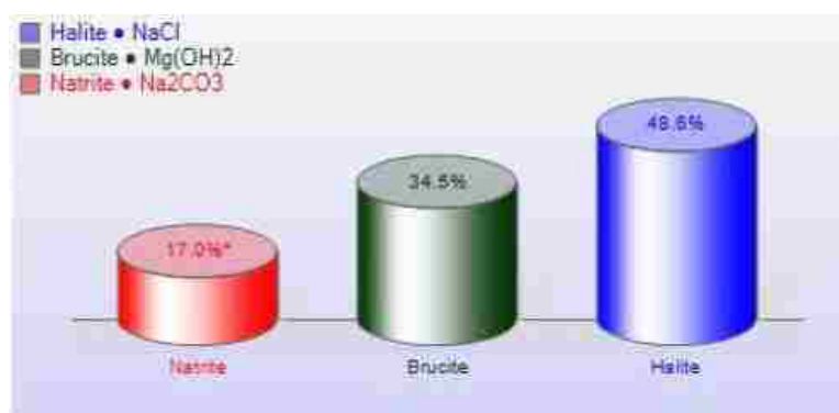
Figure 4-42: Results of XRD Analysis for Aged Mg(OH) 2
