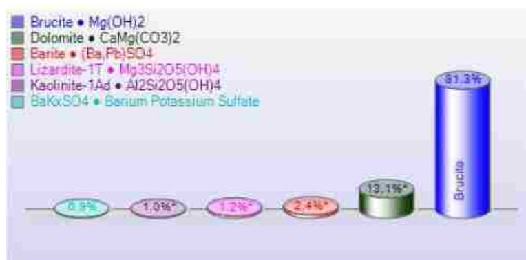
Figure 4-43: Results of XRD Analysis for Brucite
