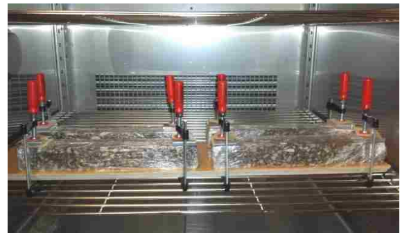
d) Applying cyclic temperature
