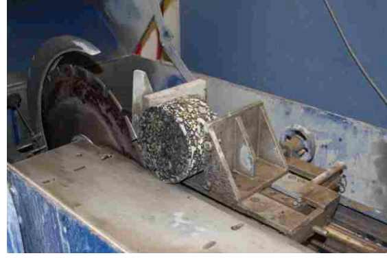
b) Sample cutting in the laboratory
