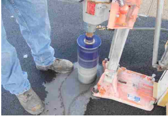
a) Collecting the field core
