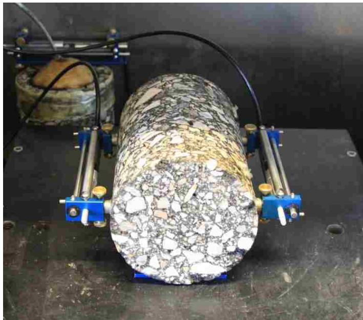
Figure 14. Measuring the thermal expansion-contraction (Vertical Direction)
