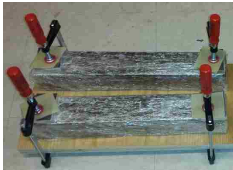
c) Restraining the samples with wood
