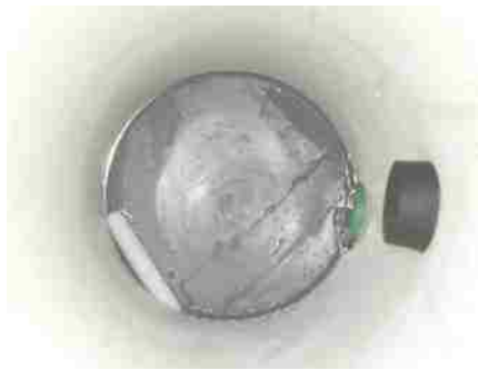
Figure 51 Stir Bar against Chamber Wall
