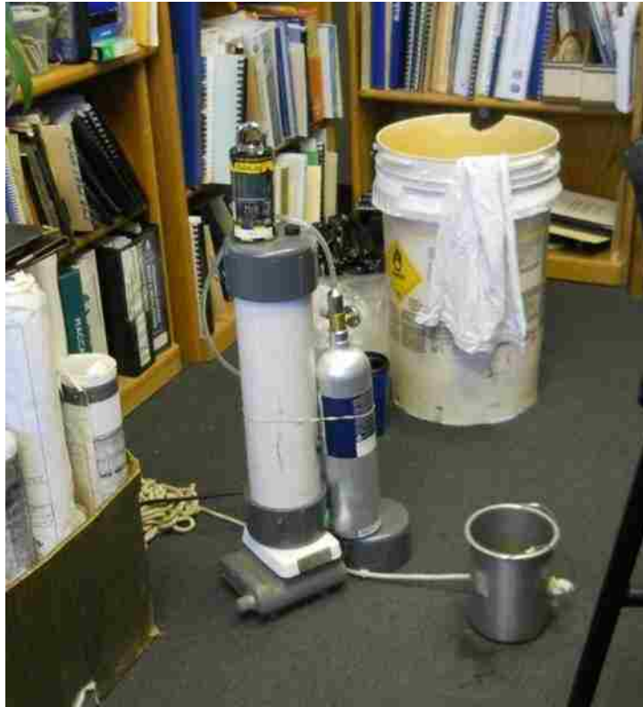
Figure 35 Office Set-Up for Dry Chamber Testing
