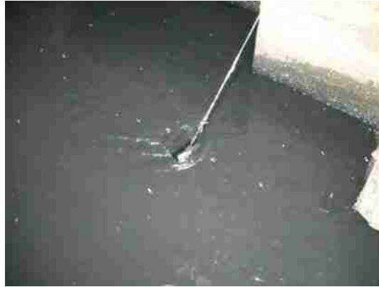
Figure 29 Sample Hanging in Effluent Channel
