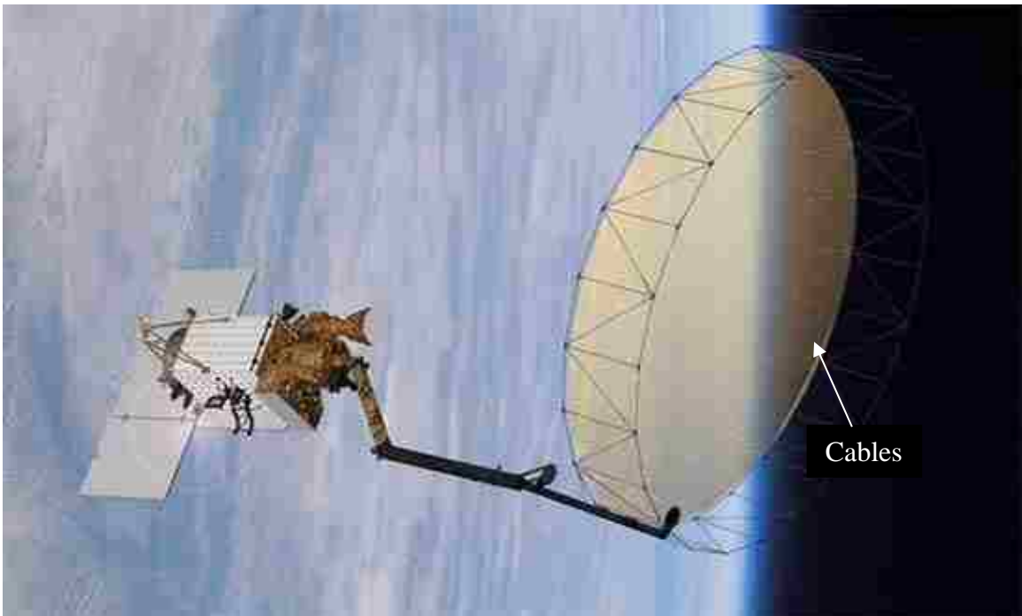
Figure 1.1.2 AstroMesh deployable satellite reflector (Northrop Grumman Corporation)
