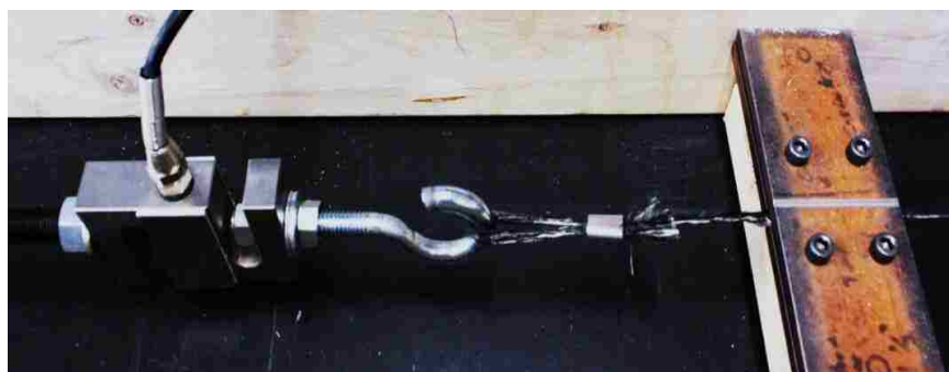
Figure 3.2.6 Connection between cable and load cell
