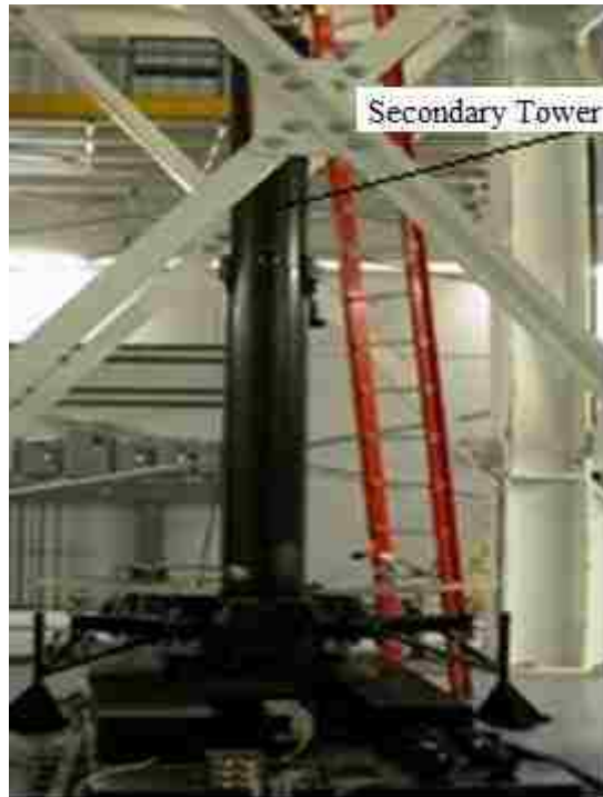
Figure 2.3.2 AFRL's Deployable Optical Telescope (Coombs et al., 2008)
