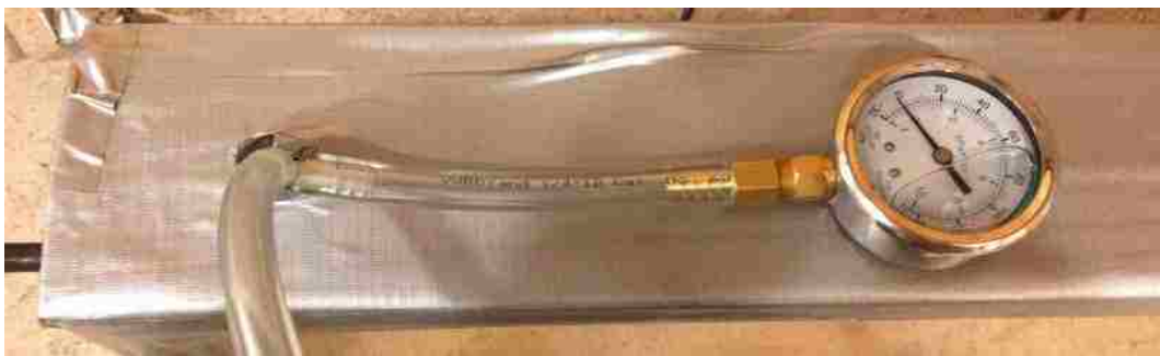
Figure 3.4.4.4 Connection between pressure gauge and chamber
