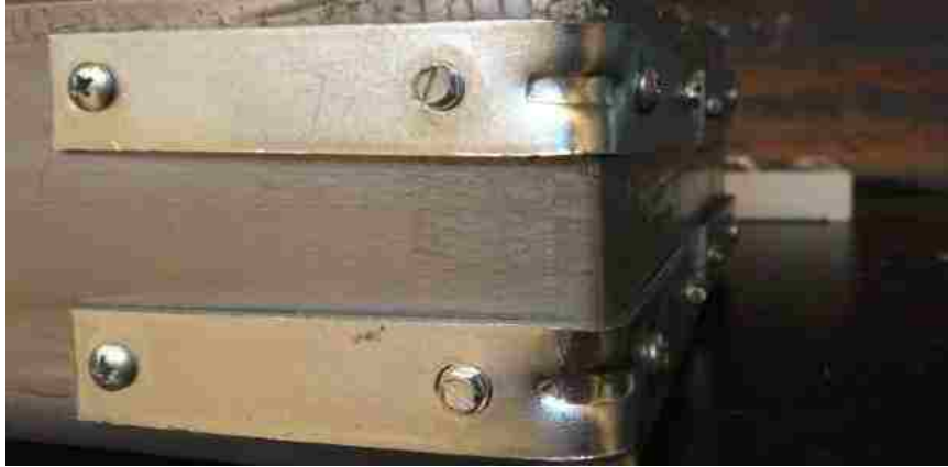
Figure 3.4.5.2 Details of the stiffened frame corners
