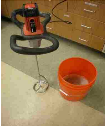
Figure 3.3 Soil Mixing in Bucket Using Mechanical Mixer
