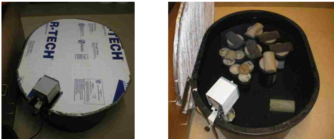
Figure 3.6 Stabilized Subgrade Soil in the Curing Tank
