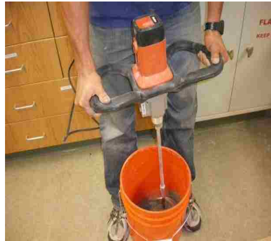
Figure 3.3 Soil Mixing in Bucket Using Mechanical Mixer
