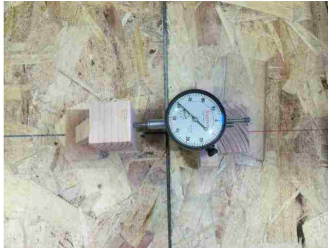
Figure 3.26 Dial gage installed at the gap discontinuity.
