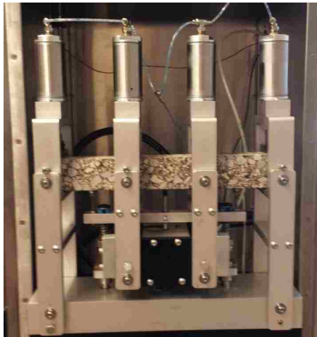
Figure 3.17: Beam Fatigue Test Setup with the LVDT Attached
