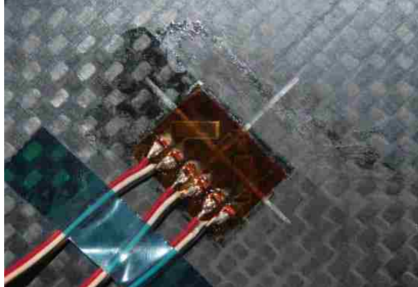
Figure 3.15: Strain gage rosette placement on PFS sample.
