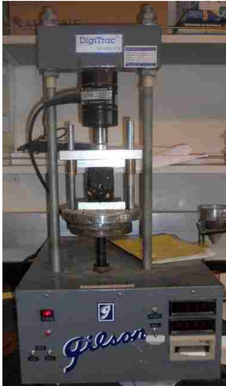
Figure 3.8 IDT testing in progress
