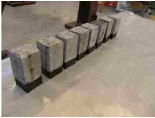
(a) Steel blocks attached to concrete substrates
