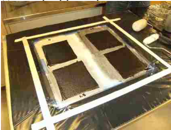
(c) Epoxy impregnated in carbon fabric
