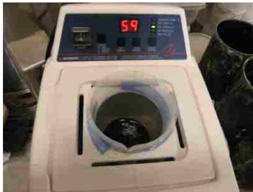
Figure 14. Ultrasonication of CNTs in epoxy resin
