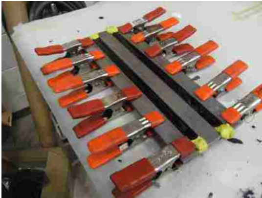
(a) Epoxy cast in steel molds
