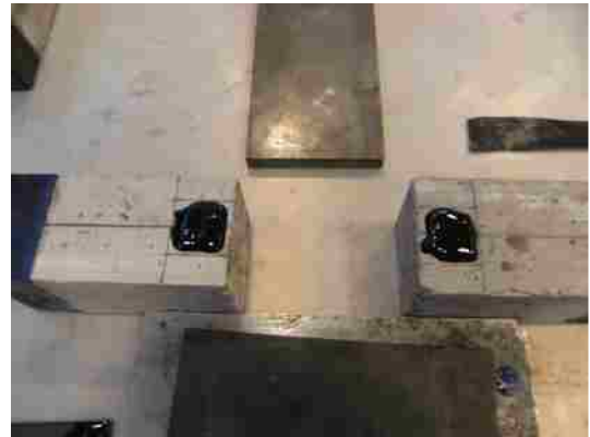
(b) Casting of CNT-epoxy composite on concrete
