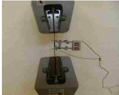
(a) Ultimate test setup for single lap shear specimen
