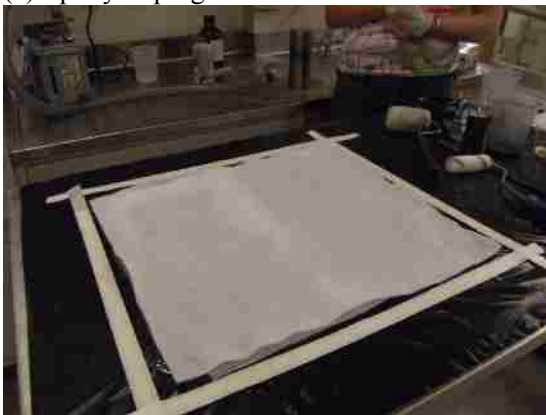
(e) Placement of breather ply
