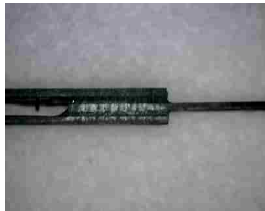
Figure 122. Double lap joint test setup (a) joint dimensions, (b) extensometer attached to the joint, (c) five specimens ready for testing, and (d) close view for the lap joint
