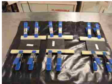
(c) Tabbing the ends using G-10 fiber glass
