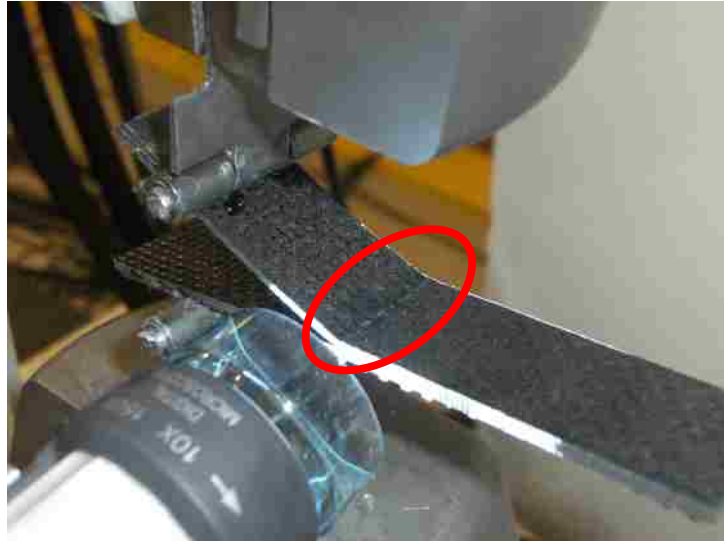
Figure 140. Flexure failure of DCB specimens
