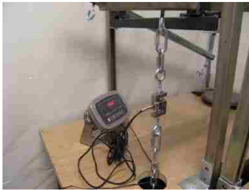
(a) Load cell attached to determine creep load
