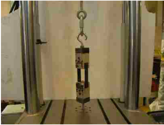
(a) Ultimate test setup for double lap shear specimen
