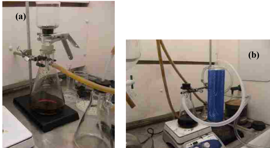
Figure 18. Filtration of functionalized CNTs
