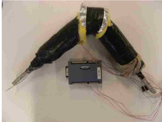
Figure 15: Thermal contact resistance specimen
