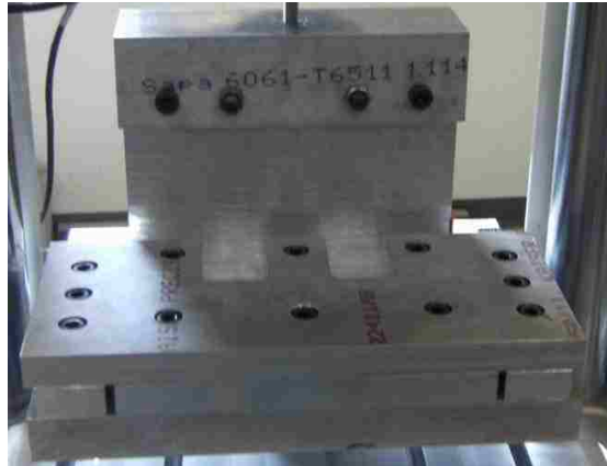
Figure 7: Test Article for measuring local shear slip
