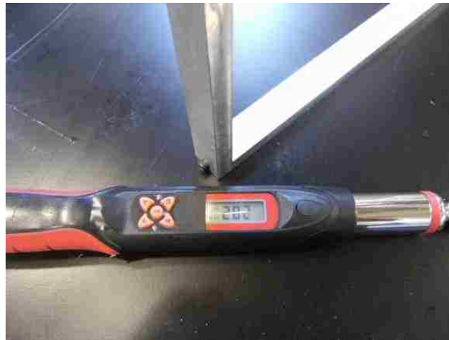
Figure 11: 90 degrees bolted joint designed and digital torque wrench
