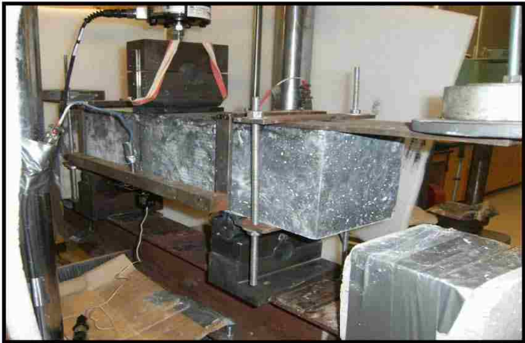
Figure 3.24: The final beam setup for starting the test
