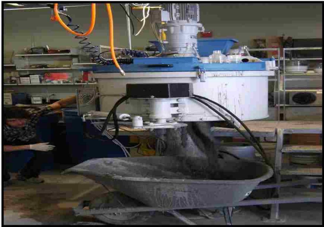
Figure 3.2: The final mix exiting the mixer
