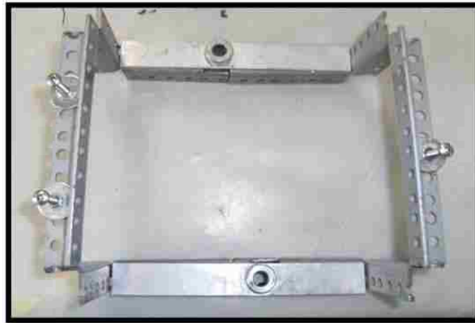
Figure 3.18: Frame for the smaller size of beams
