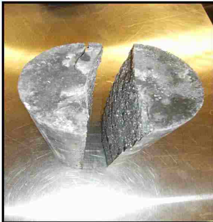
Figure 3.5: The UHPC specimen after the split tension test
