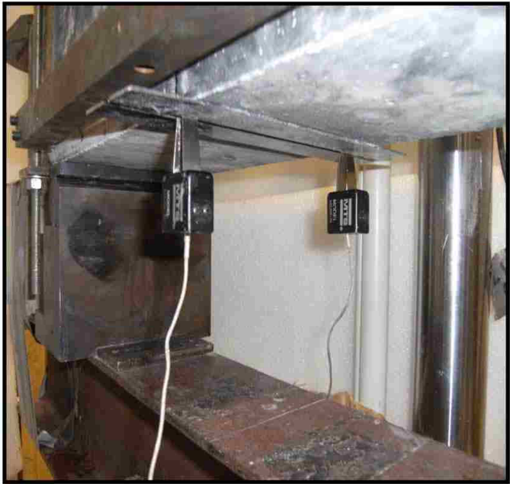
Figure 3.22: Attachment of clip gages to the knives
