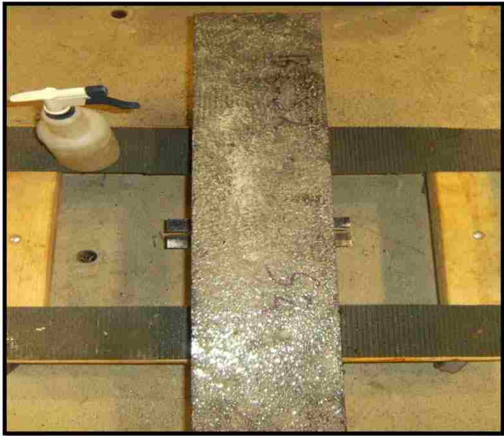
Figure 3.21: The attachment of knives to specimen with the super glue, and keeping of the specimen wet by water spray
