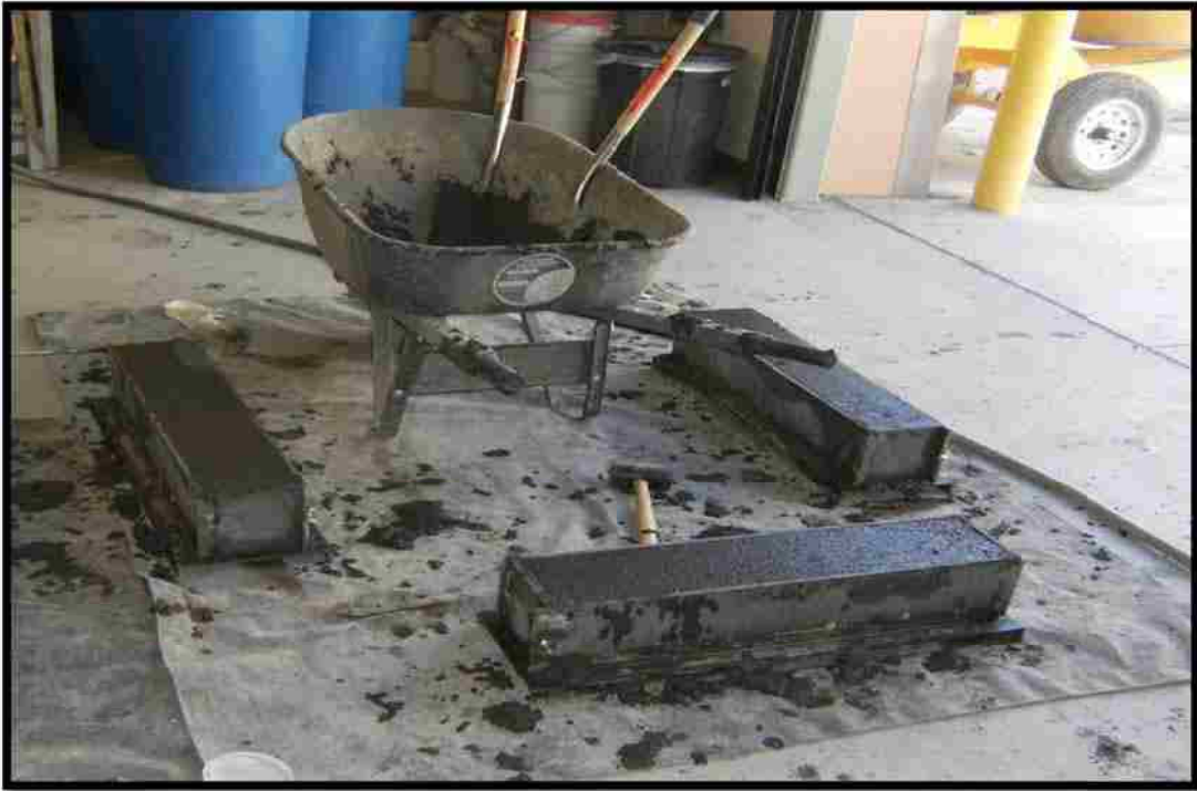
Figure 3.3: The specimens after the screeding
