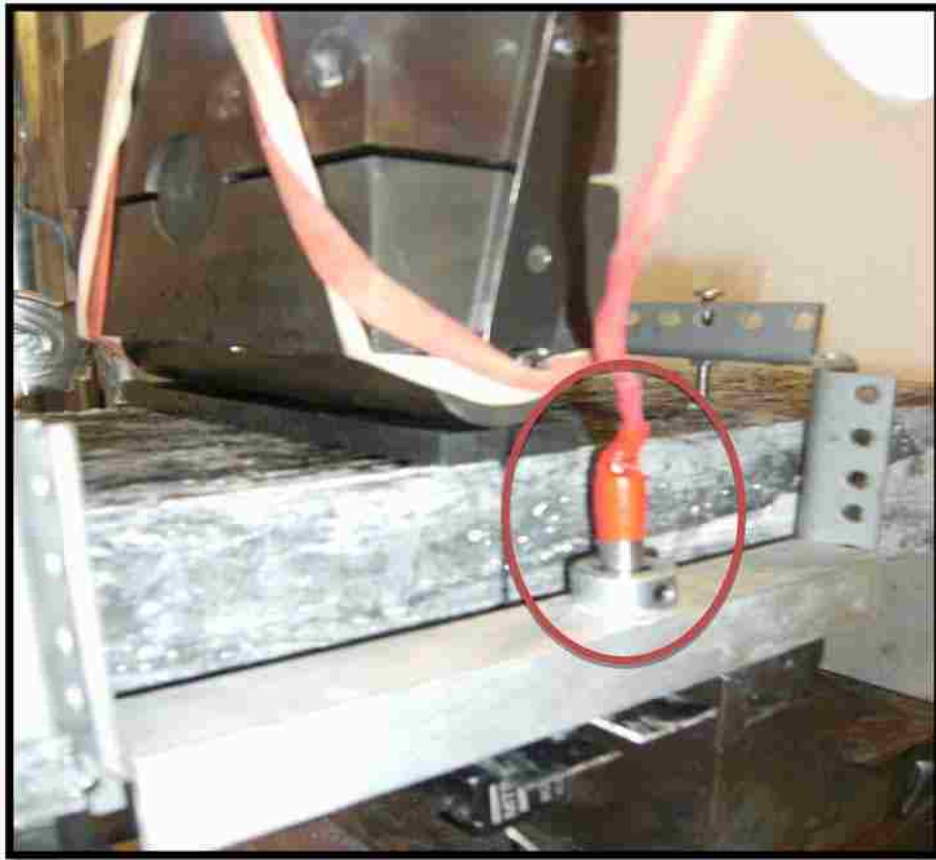
Figure 3.23: Placement of LVDTs in the frame
