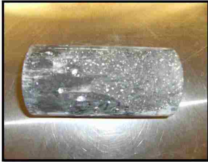
Figure 3.4: The UHPC specimen after the compression test
