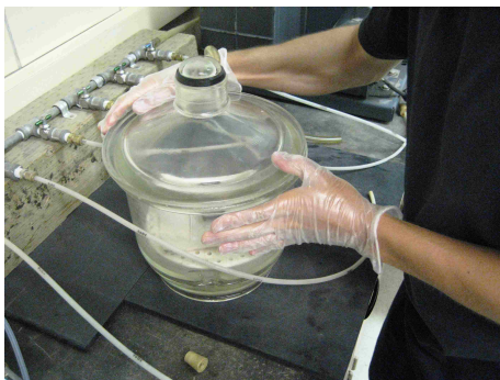
Figure 3.6: Picture of elastomer specimen in vacuum chamber
