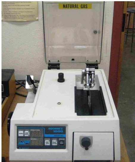
Figure 3.8: Isometric saw used to cut specimens
