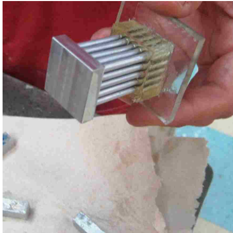
Figure 3.10: Picture of epoxy specimen being removed from greased L-Clamps
