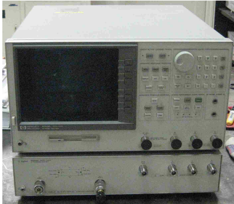
Figure 3.14: Picture of network analyzer and S-parameter test set
