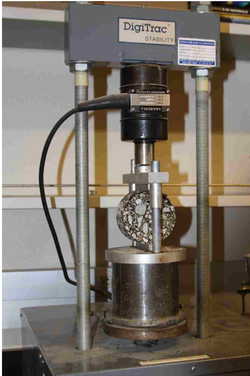
Figure 4.2. IDT Testing Apparatus
