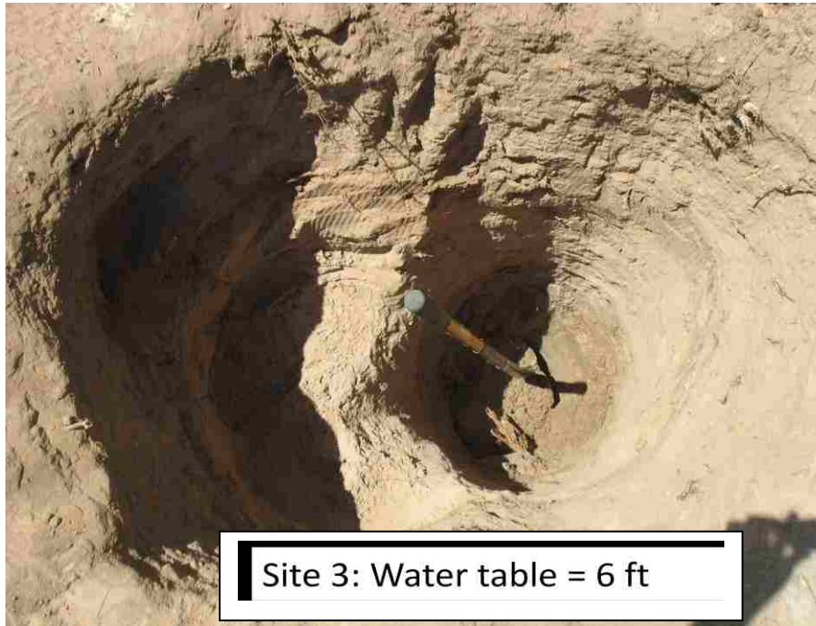
Figure 27. The hole that was dug at site 3
