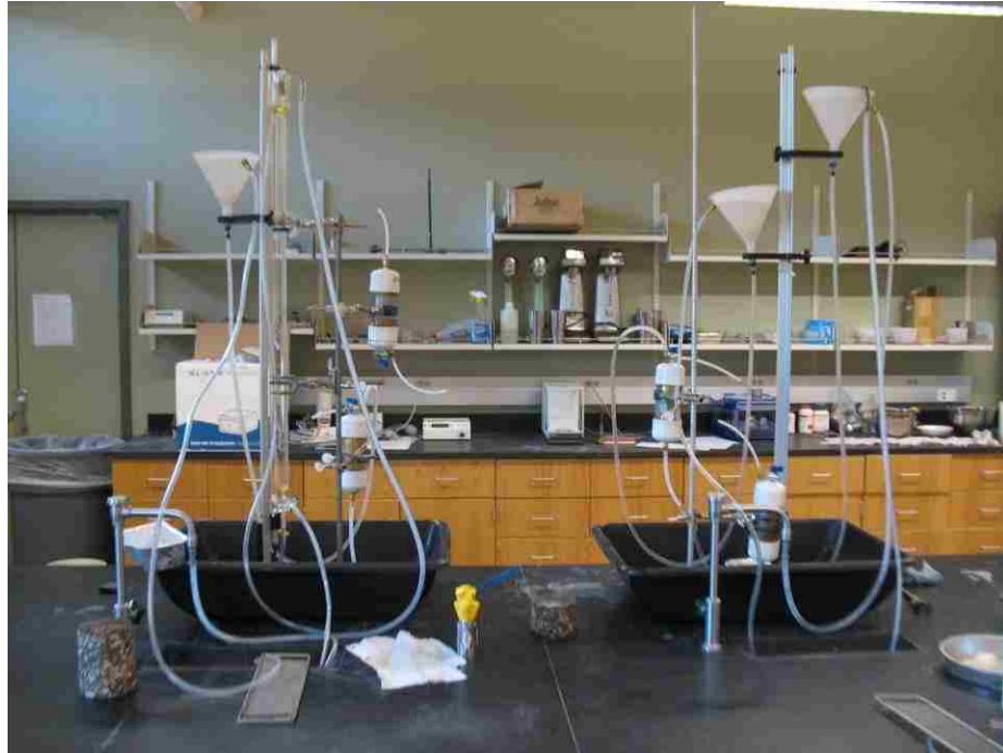
Figure 33. Constant head (right) and falling head (left) hydraulic conductivity apparatus
