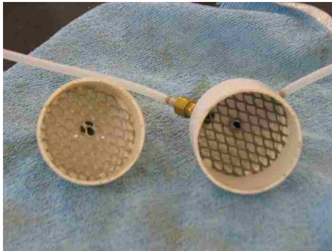
Figure 32. Caps used for the hydraulic conductivity samples. Screens restricted swelling of sample during saturation
