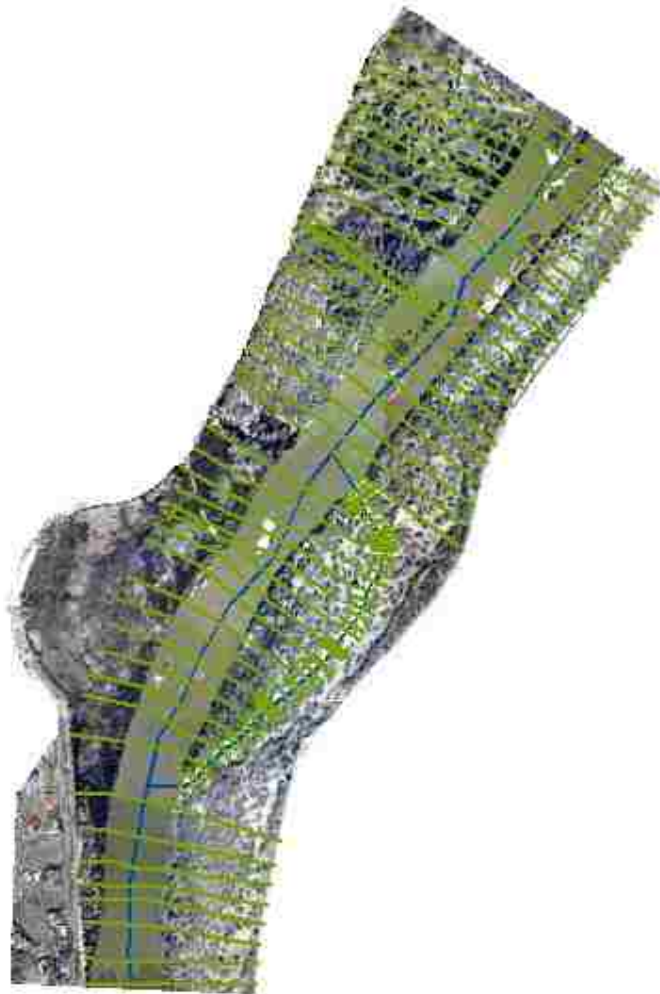
Figure 3-2: Plan View of Second HEC-RAS Model Geometry
