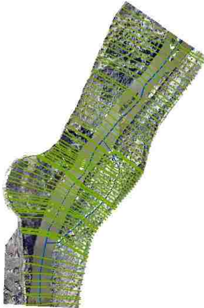
Figure 3-1: Plan View of First HEC-RAS Model Geometry
