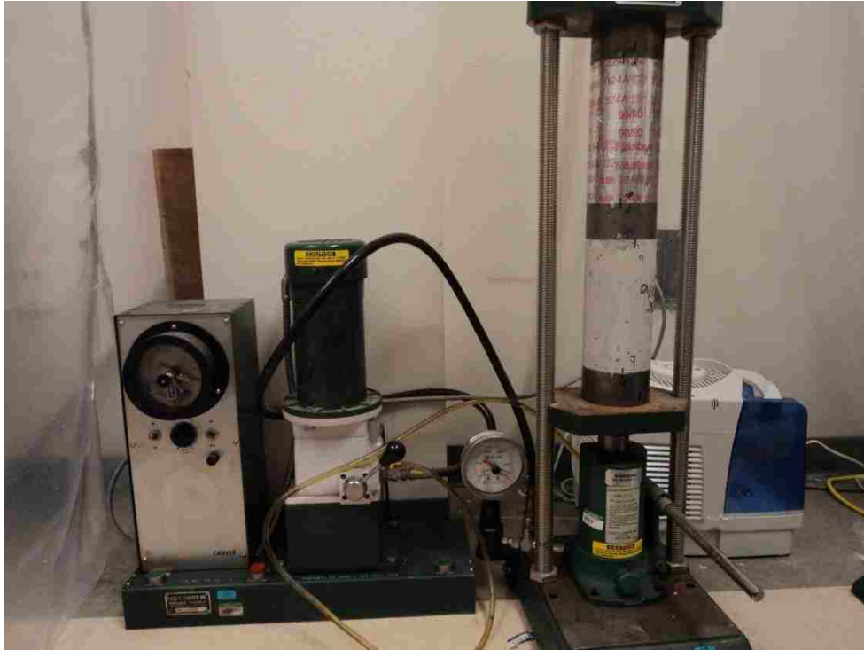
Figure 3.10 – Creep test in progress utilizing creep frame
