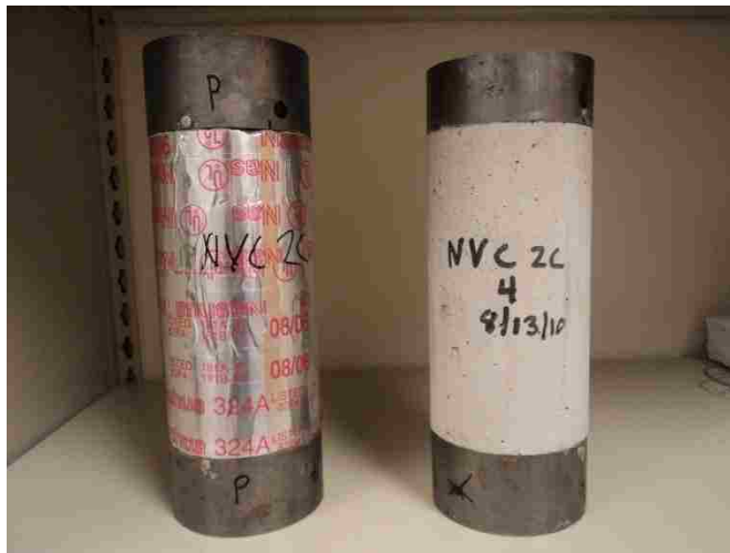
Figure 3.12 – Creep specimen preparation
