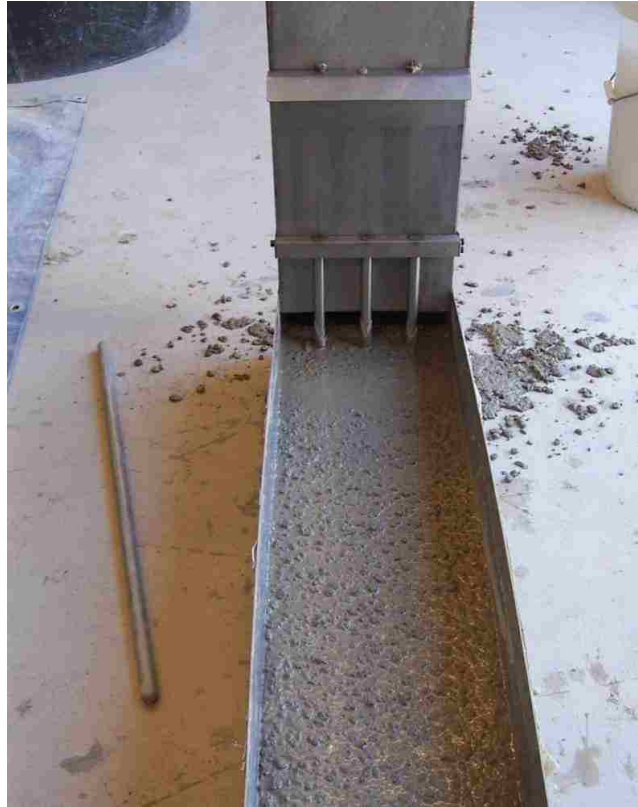
Figure 3.7 – L-Box test to determine SCC passing ability
