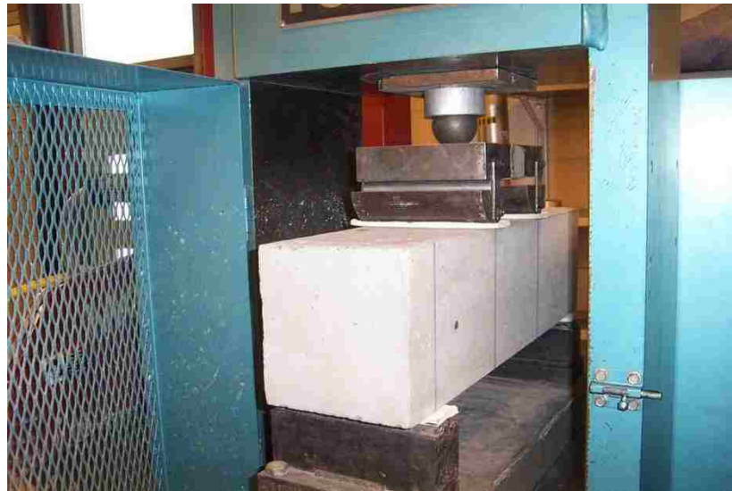
Figure 3.8 – Modulus of rupture testing
