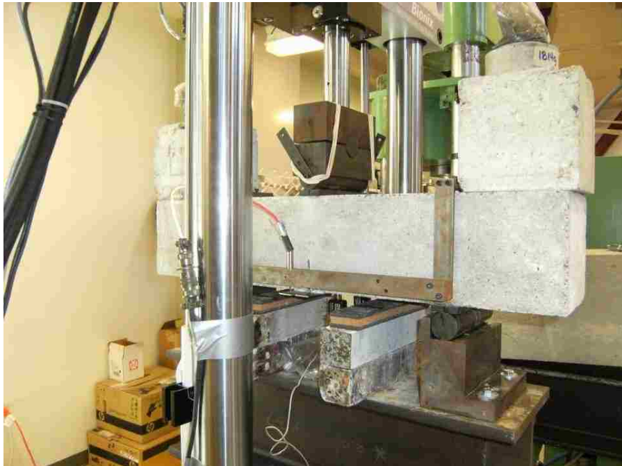
Figure 3.15 – Test setup with counterweights
