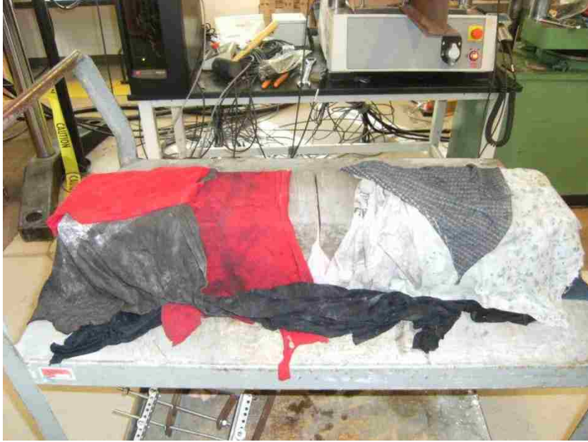
Figure 3.14 - Transporting beam to not allow drying
