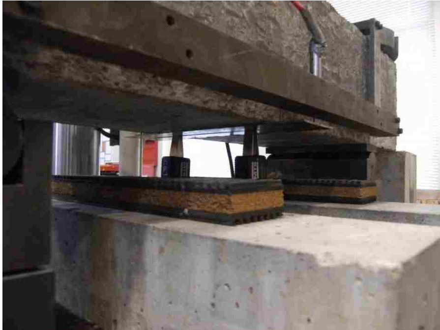
Figure 3.16 – Installation of clip gages
