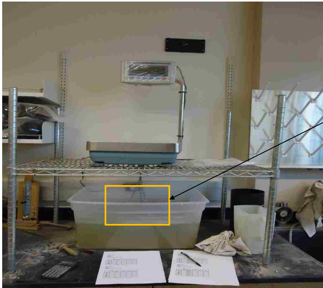
Figure 6.5 A part of laboratory setup for measuring G_{mb}
