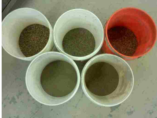
Figure 36: Proportioned aggregate for making mortar sand.
