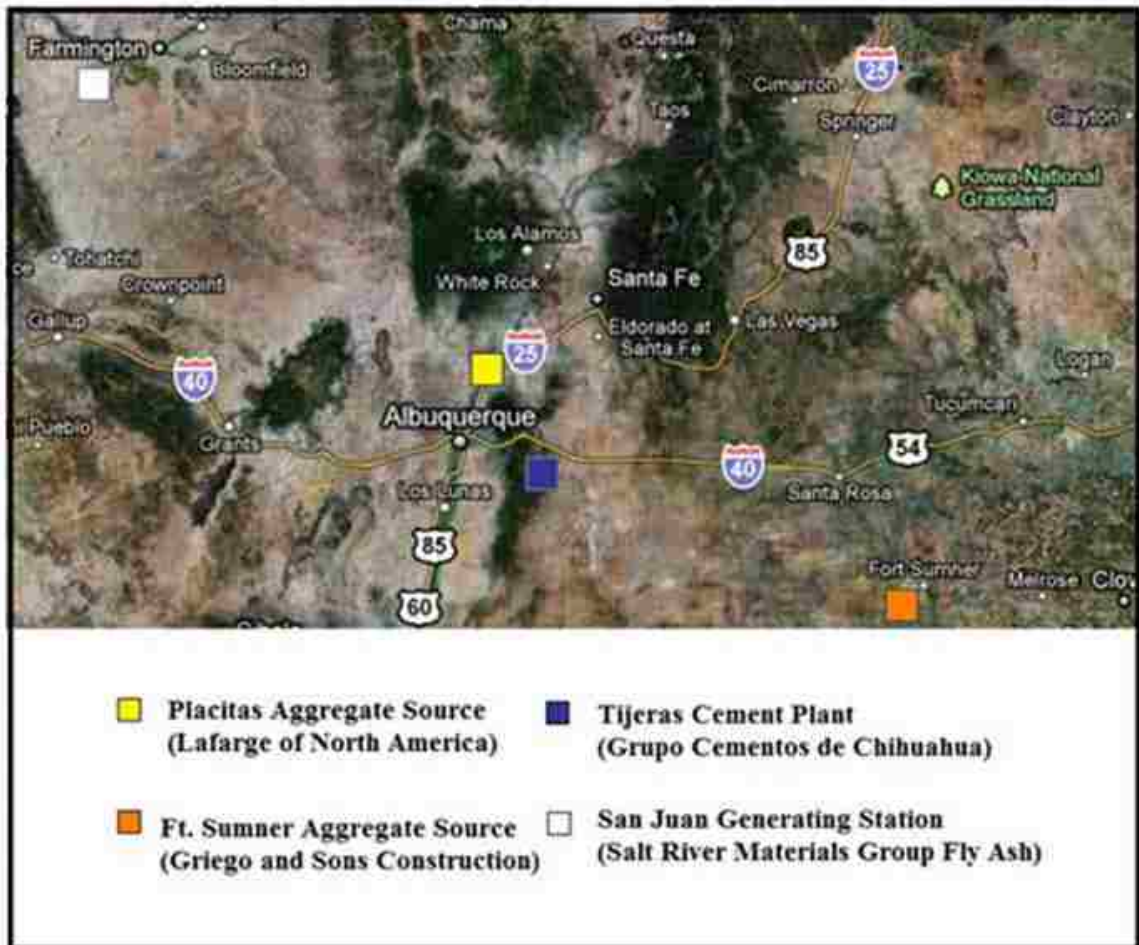
Figure 10: Locations of New Mexico’s concrete material sources
