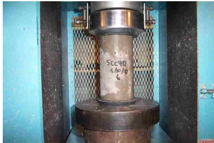
Figure 24: Compression of a 4" x 8" cylindrical concrete specimen.
