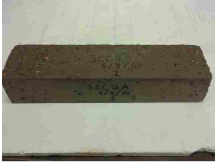
Figure 34: Prismatic specimen exposed to 108 freeze thaw cycles
