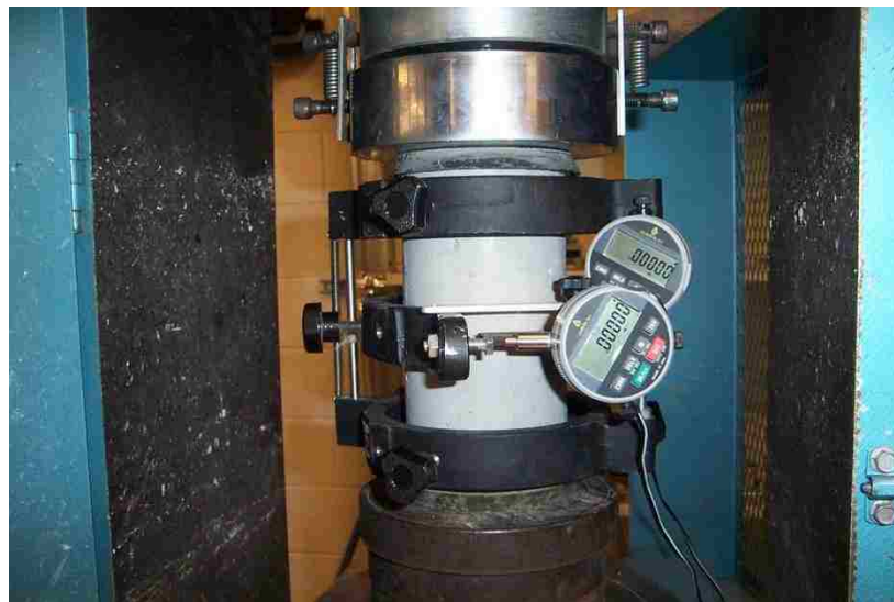
Figure 26: Compressometer and cylinder assembly used to measure static modulus of elasticity and Poisson's ratio
