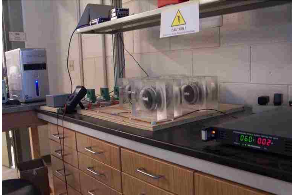
Figure 30: Rapid Chloride Ion Penetration test on SCC.
