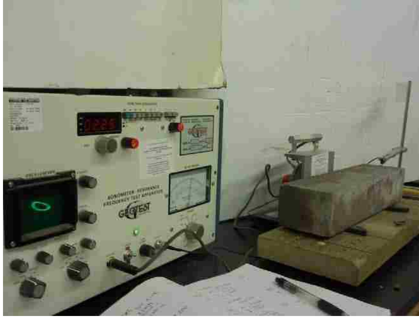
Figure 35: Prismatic concrete specimen positioned to determine transverse resonant frequency.
