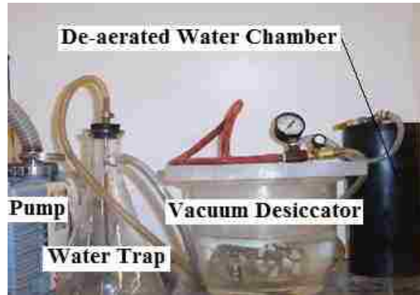
Figure 28: Schematic of Vacuum Desiccator
