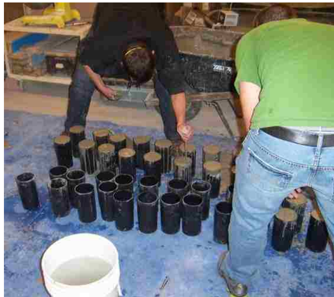
Figure 23: Casting 4" x 8" cylindrical concrete specimens.
