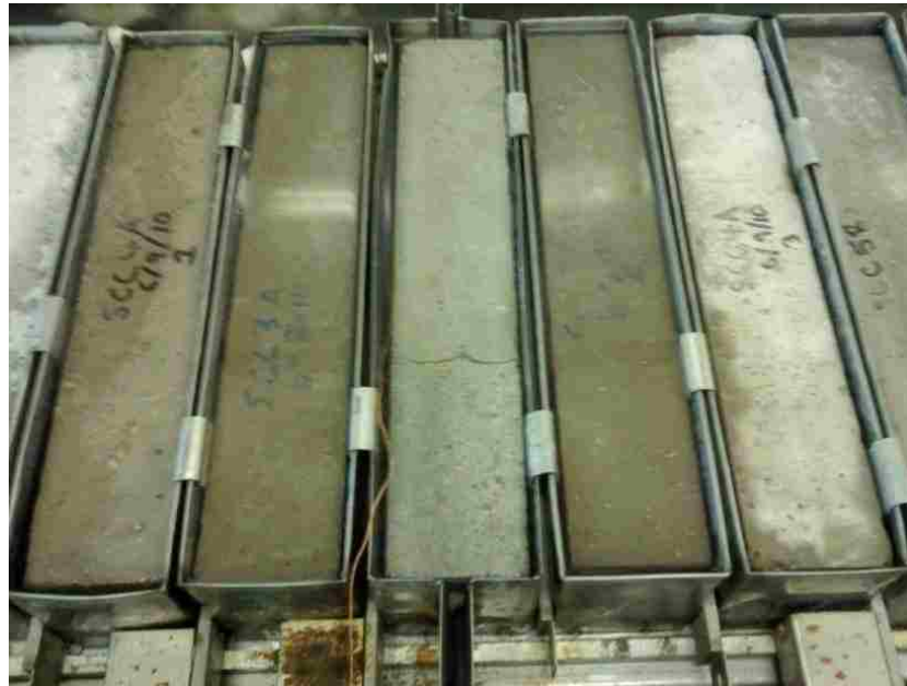
Figure 32: SCC specimens placed in freeze-thaw apparatus.
