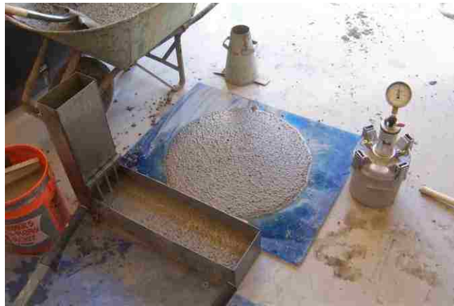
Fig 21: L-box, slump flow, and air pressure meter to test fresh properties of SCC.
