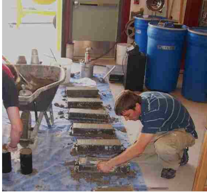
Figure 22: Casting 4" x 3" x 16" prismatic concrete beams.
