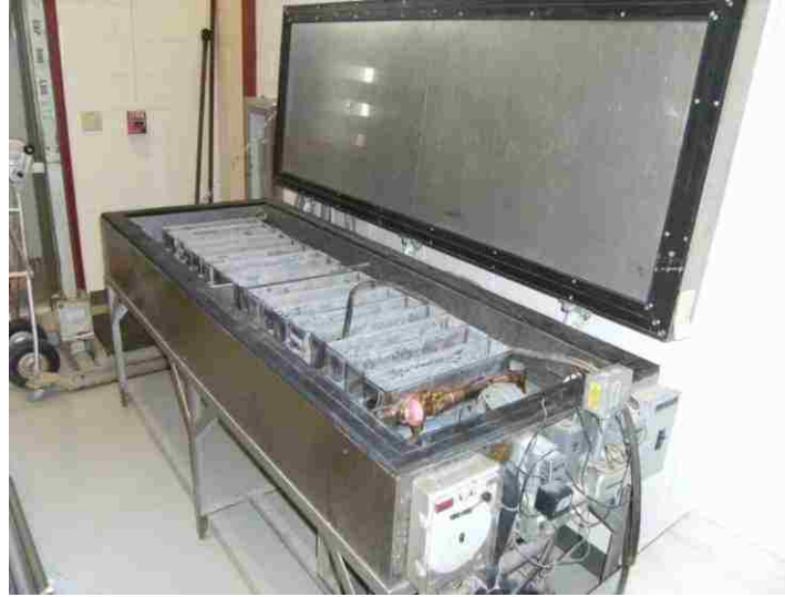
Figure 31: Freeze-thaw equipment to test freeze-thaw resistance of SCC.
