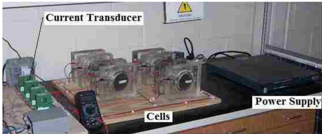
Figure 29: Rapid chloride ion penetration device.
