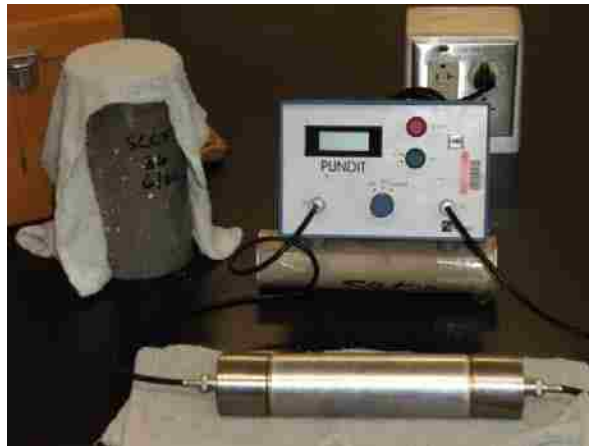
Figure 27: Pulse velocity apparatus
