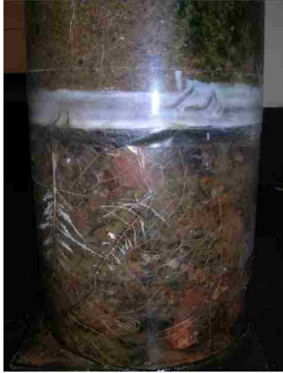
Figure 3.9 Picture of root system grow found outside of the column
