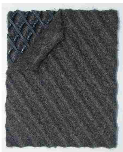
Figure A-2 Geocomposite
