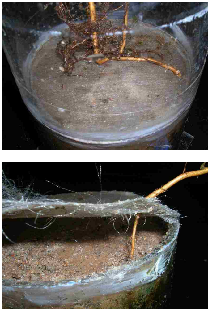
Figure 3.4 Photograph of root growth through geotextile
