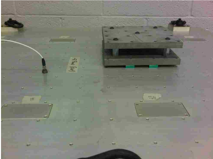
Figure 4.8: Photo of Mock Satellite Test Setup with Mass Attached
