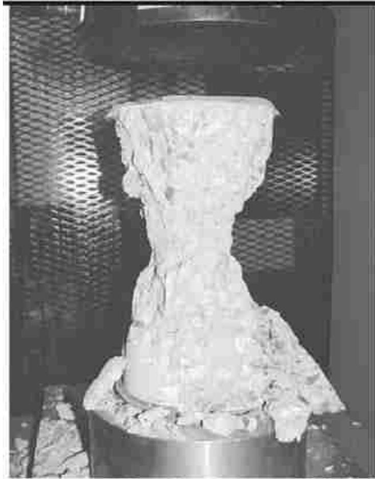
Fig. 4.6 Concrete specimen failed in compression test.
