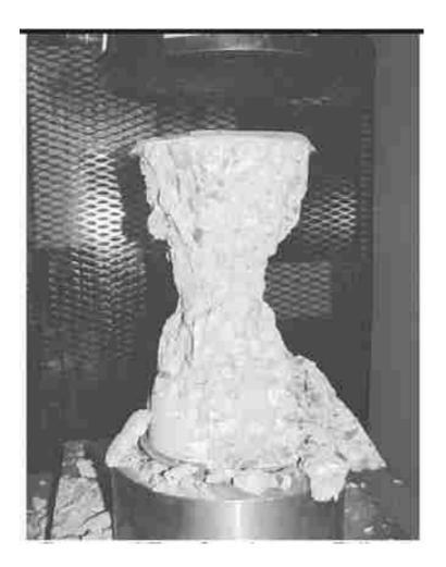
Fig. 4.6 Concrete specimen failed in compression test. [NRMCA, 2003]
