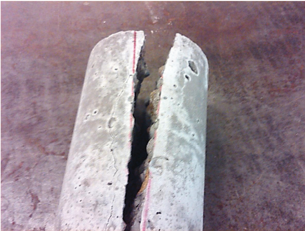
Figure 20: Splitting tensile test specimen
