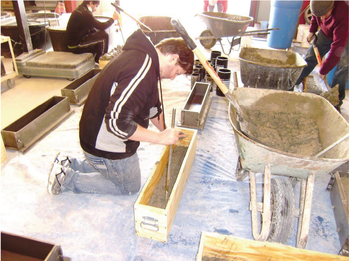
Figure 19: Casting of beam specimens
