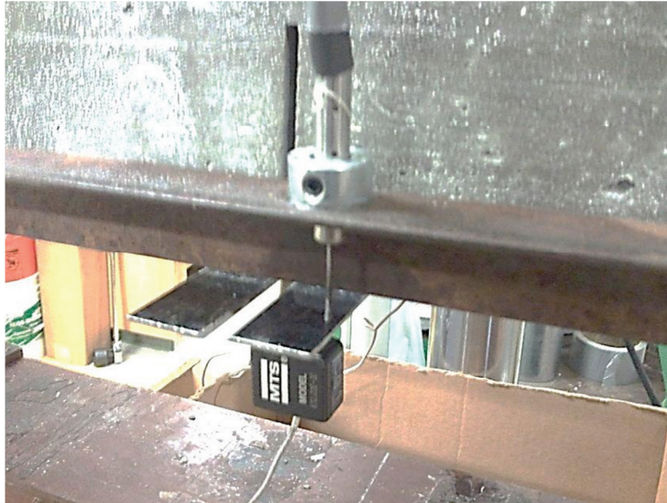
Figure 35: Photograph of LVDT attached to reference frame, resting upon knife edge
