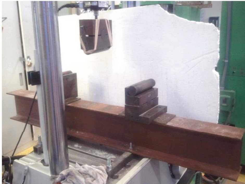
Figure 26: Photograph of support beam
