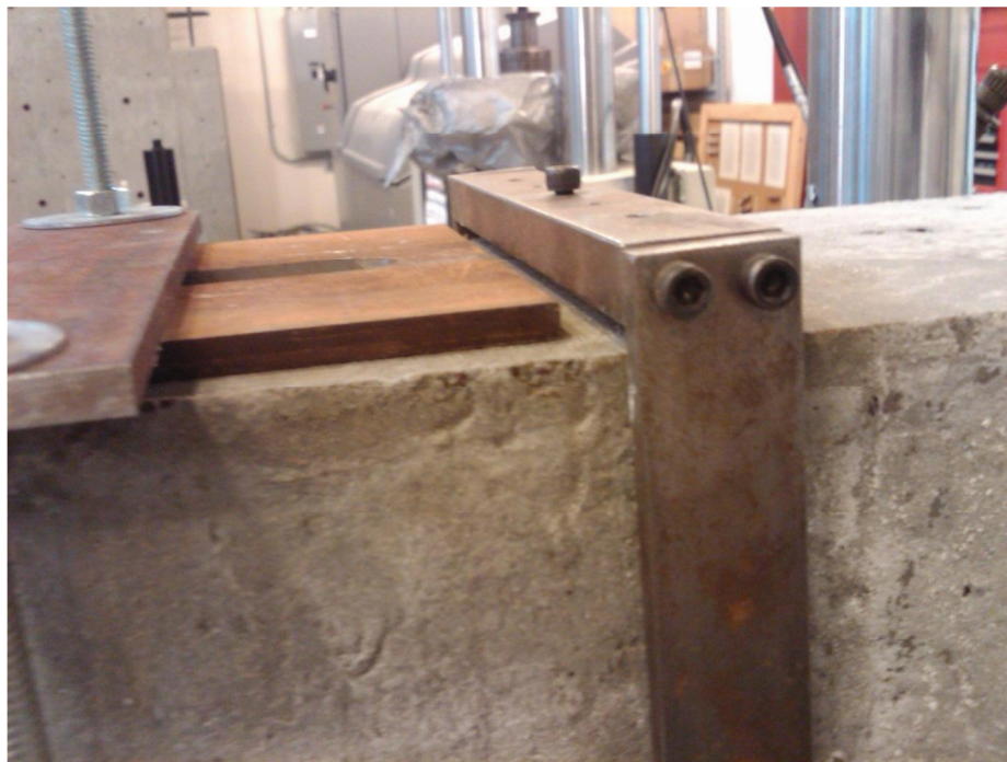
Figure 33: Detail showing counterweight holding plate does not interfere with LVDT reference frame
