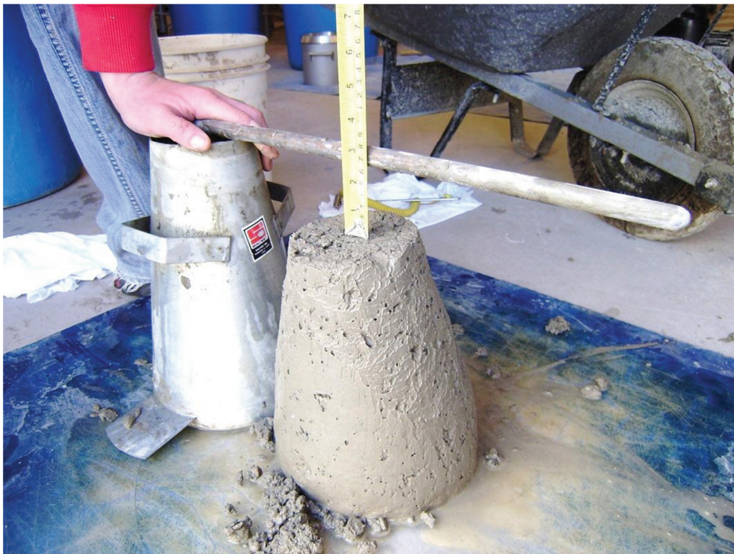
Figure 18: Concrete slump on day of casting
