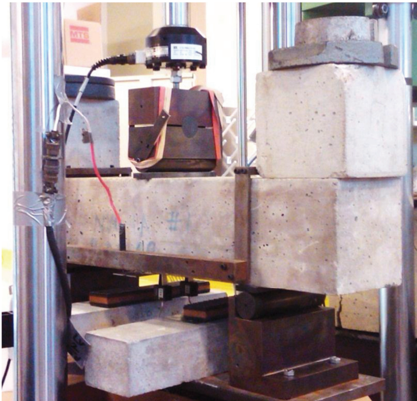
Figure 30: Dummy specimen with stacked counterweights on overhangs
