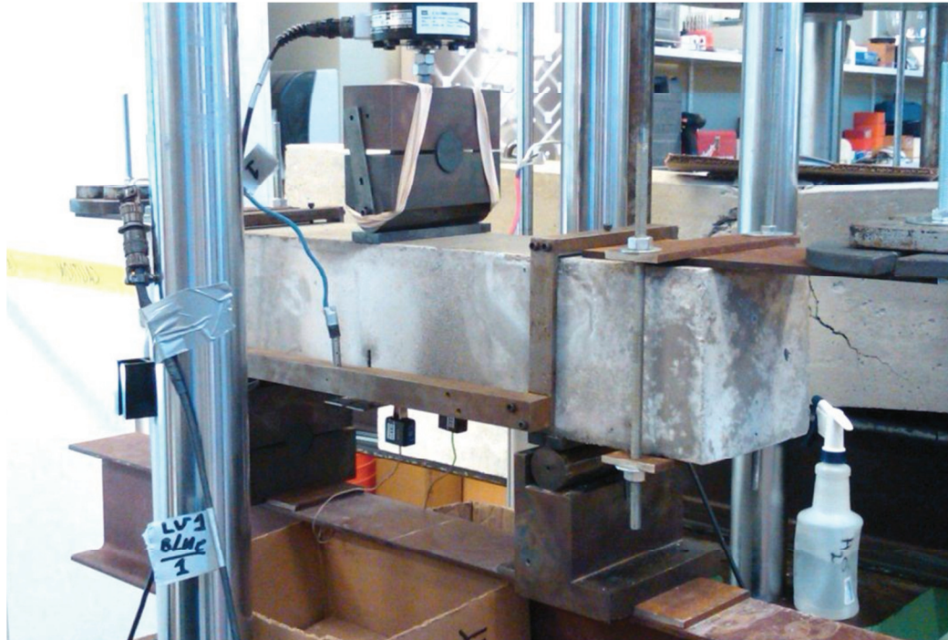
Figure 28: Setup for 152 mm (6 in) deep beam
