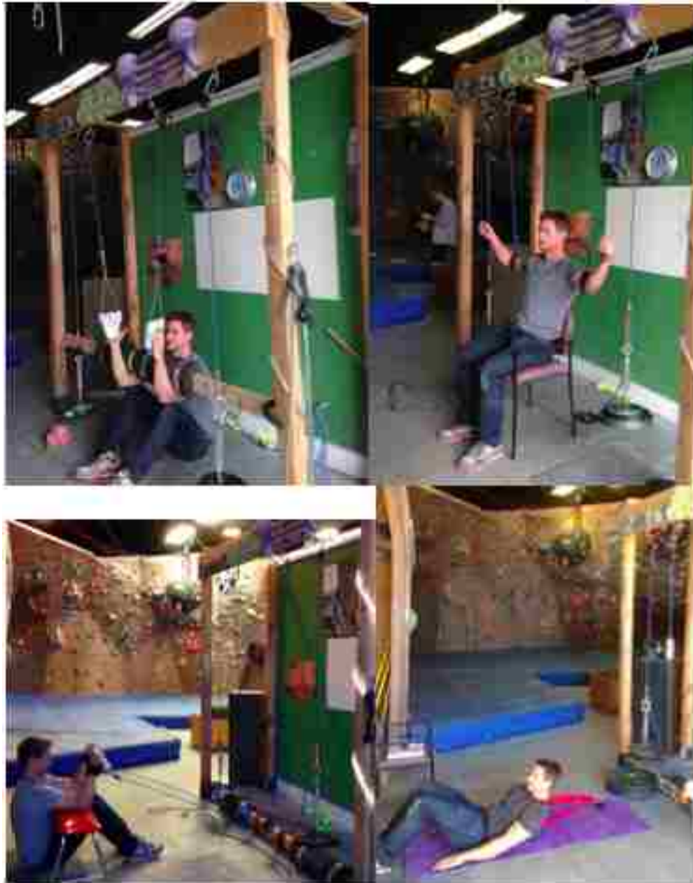
Figure 5. This figure shows the weighted rope and pulley systems for each pre-fatiguing exercise. Clockwise from top left: digit flexion apparatus, shoulder adduction apparatus, elbow flexion apparatus, and lumbar flexion apparatus.
