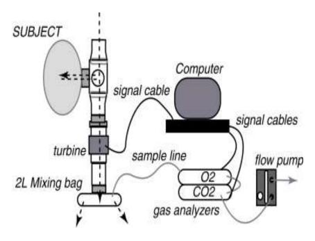
Figure 15. Schematic of the custom developed system for EGAIC.
