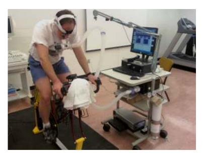
Figure 17. The subject exercising with analyses performed by the commercial (ParvoMedics) system for hypothesis 3 testing.
