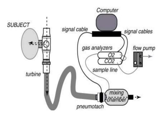
Figure 16. Schematic of the commercial (ParvoMedics) EGAIC system.
