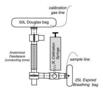
Figure 6. Schematic of the equipment set-up for hypothesis 1 testing for the 25 L expired breathing (Douglas) bag condition without the added low resistance tubing.
