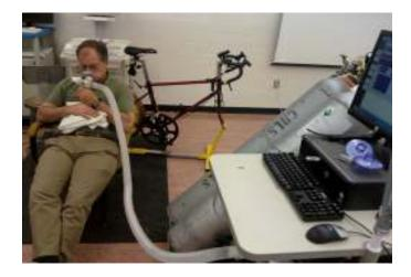
Figure 14. Photograph of the commercial (ParvoMedics) EGAIC system during the rest condition.
