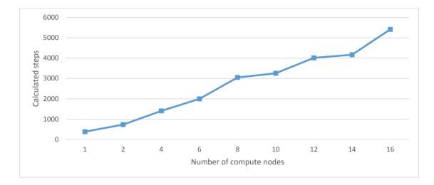
Figure 5.55: XFLAT heterogeneous multi-node performance on Stampede (one CPU and one MIC per node) for various numbers of compute nodes. The calculated radial steps were measured for a  $\sim 100$  second run.
