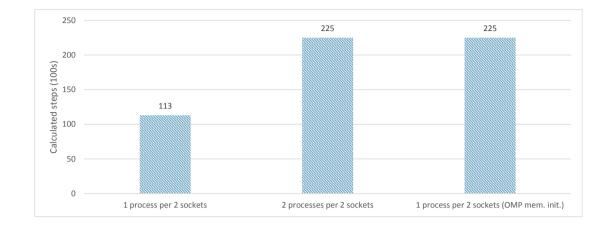
Figure 5.27: Performance of three alternative methods of running XFLAT on a NUMA system (Stampede). The calculated radial steps were measured for 100-second runs. From left to right, one XFLAT instance employed the entire dual-socket node, two XFLAT instances each employed a single CPU socket, and one XFLAT instance initialized memory in parallel and employed the entire dual-socket node. Net computed radial steps (listed at the top of the bars) were measured for  $\sim 100$  second runs.
