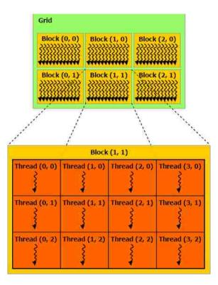
Figure 2.4: Grid of thread blocks. A grid (shown in green) may contain a multidimensional array of blocks (shown in yellow). Within each block there is an array of threads (shown in orange) (Figure from NVIDIA 2014).
