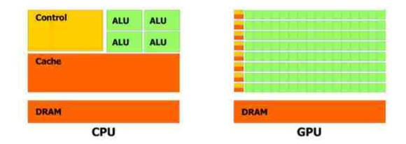
Figure 1.5: Comparison of the CPU and GPU die area. The CPU has more on-chip memory (shown in orange) and larger control unit (shown in yellow) than GPU. However, the GPU devotes more transistors to data processing (shown in green) than CPU [NVIDIA, 2012a].
