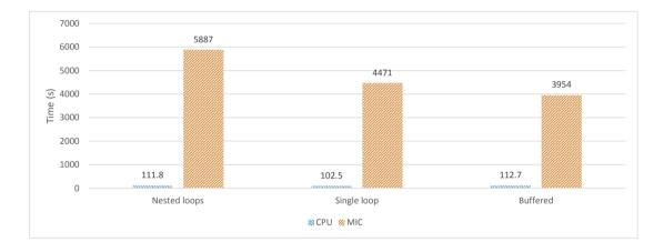
Figure 5.32: XFLAT's I/O performance on the CPU and MIC for three different approaches on Stampede. The performance of the MIC (orange bars) was 35 to 53 times worse than the performance of CPU (blue bars). Numbers at top of bars correspond to time in seconds.
