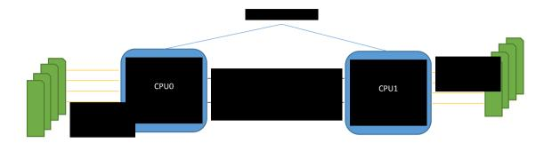
Figure 5.48: A single MPI task per node that employs the entire system including all available processors on the NUMA architecture. Blue squares are CPUs and green recangles are RAM modules.
