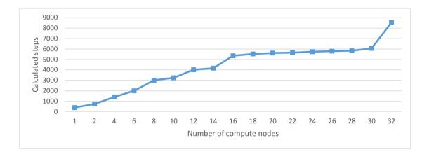
Figure 5.61: XFLAT heterogeneous multi-node performance on Stampede (one CPU and one MIC per node) employing up to 32 nodes. The calculated radial steps were measured for about  $\sim 100$  second run.
