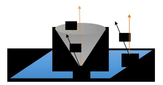
Figure 3.5: Illustration of the plane geometry. The point  $p_0$  and  $p_1$  have identical neutrino emission. For every zenith angle  $\vartheta$ , there are multiple neutrino trajectories along different  $\varphi$  angles (shown as the grey cone).
