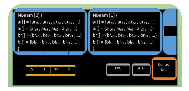
Figure 4.6: Within a processor core (green), NBeam objects can employ the lowest level of parallelism, SIMD unit (shown in yellow). Each NBeam instance (shown in blue) issues vector instructions in order to utilize SIMD unit.
