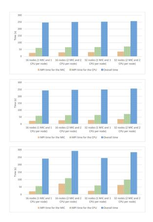
Figure 5.82: Performance of the old style algorithm (top panel), the reordered algorithm (middle panel), and the new style algorithm (bottom panel). There were six MPI function calls per loop iteration. The orange bar shows the maximum MPI time among the MICs' processes, the green bar shows the maximum MPI time among the CPUs' processes, and the blue bar shows the overall run time in seconds.
