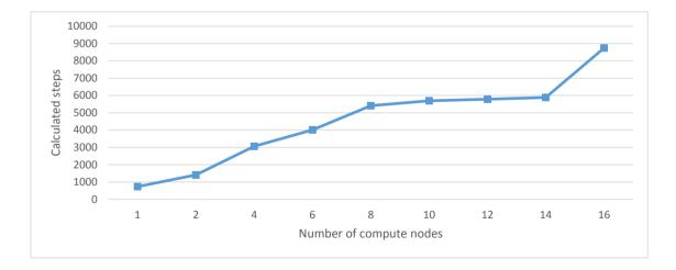
Figure 5.59: XFLAT heterogeneous multi-node performance on Stampede (two CPUs and two MICs per node) for various numbers of compute nodes. The calculated radial steps were measured for  $\sim 100$  second run.
