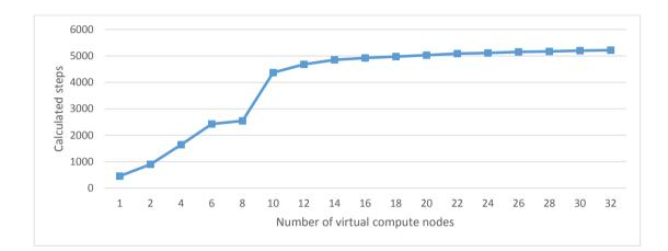
Figure 5.70: Simulated multi-node benchmark on single node (one CPU and one MIC) of Stampede. At each point, the load on the node was adjusted to be equal to the load on a node in a multi-node configuration. The benchmark employed different problem sizes  $(3000 \times 30 \times 100 \text{ beams})$  and the 2.9:1 MIC to CPU load ratio. The number of calculated radial steps was measured for about ~ 100 seconds.
