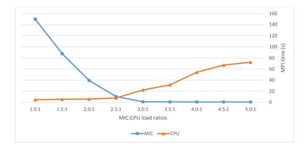
Figure 5.73: Measured MPI communications time for XFLAT on Stampede as the function of MIC to CPU load ratio. The problem size was set to  $5550 \times 10 \times 100$ , the code was run for 1k radial steps, and the run time were measured in seconds.
