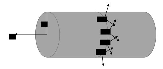
Figure 3.6: Illustration of the cylinder model and its emitting points' trajectories. Neutrinos emitting from points  $p_1$ ,  $p_2$ ,  $p_3$ , and  $p_4$  are different; however, since azimuthal symmetry is assumed, points located along the z axis are all identical. r is the radius of the cylinder.
