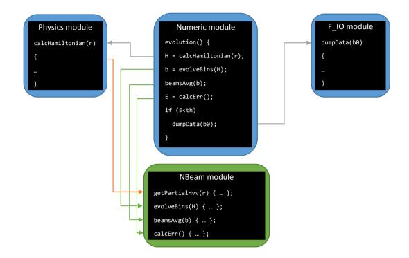
Figure 4.13: Function dependency between modules and the order of the function calls. Upper layer modules are shown in blue, and bottom layer modules are shown in green.
