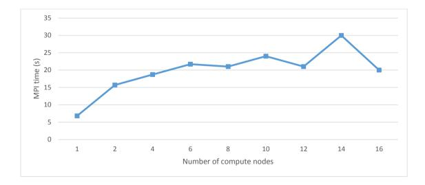
Figure 5.56: Maximum spent time within MPI functions for various numbers of nodes on Stampede (using one CPU and one MIC per node). The problem size was set to  $10000 \times 10 \times 100$  beams and the number of processed radial steps was measured over  $\sim 100$  second period of run time.
