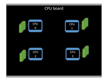
Figure 4.19: Non-Uniform Memory Access architecture. The memory (shown in green) connected to a particular CPU (shown in blue) is visible and accessible by threads on other CPUs through the QPI link (black lines).
