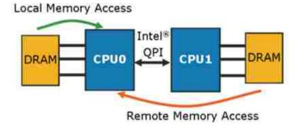
Figure 4.20: Illustration of accessing the memory (shown in yellow) in multi-socket CPU (shown in blue) architecture and the impact on the thread performance due to the route to the memory [SlideShare, 2015].
