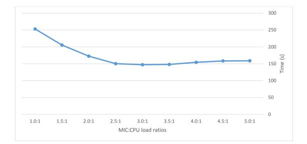
Figure 5.72: XFLAT overall run time on Stampede as the function of MIC to CPU load ratio. The problem size was set to  $5550 \times 10 \times 100$ , the code was run for 1k radial steps, and run time was measured in seconds.
