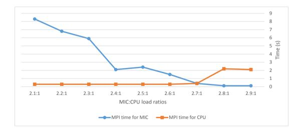
Figure 5.78: XFLAT timing behavior when the fourth section of the code including the third MPI reduction was benchmarked. The blue curve shows the measured time of MPI invocation on the MIC side, and the orange curve shows the measured time of MPI invocation on the CPU side.
