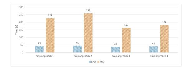
Figure 5.25: Illustration of CPU (blue bars) and MIC (orange bars) OpenMP performance on Stampede for  $1M \times 1k$  loop iteration counts (outer\_loop\_len  $\times$  inner\_loop\_len). Numbers on top of bars correspond to total time in seconds.
