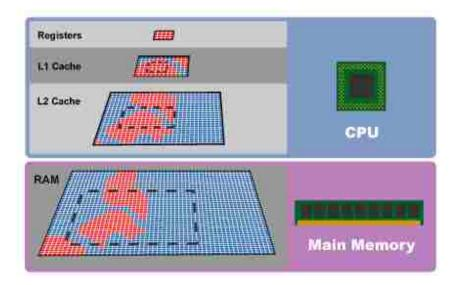
Figure 4.22: Caching pyramid illustration. For each memory fetch, the CPU fetches a region of memory containing the required data. If a particular memory location is referenced at a particular time, then it is likely that nearby memory locations will be referenced in the near future [ArsTechnica, 2015].
