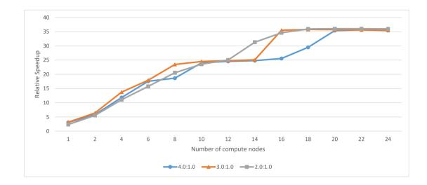
Figure 5.1: XFLAT speedup relative to single node (CPU only) on a multi-node environment. The blue, orange, and grey curves correspond to MIC to CPU load ratios of 4:1, 3:1, and 2:1, respectively.
