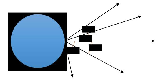
Figure 3.3: Illustration of multi-zenith angle model. There are different trajectories along zenith direction  $(\vartheta_1, \vartheta_2, \vartheta_3, \vartheta_4)$  emitted from a single point on the star's surface (shown in blue), and every point on the surface is assumed to be equivalent.
