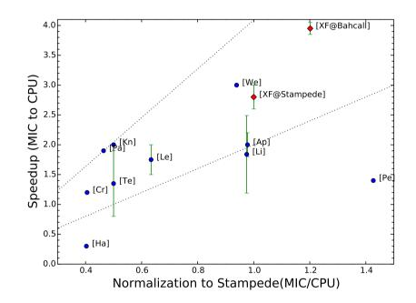
Figure 2.14: Illustration of the relative MIC to CPU speedup of different applications. The x-axis is the  $MIC's\ cores \times MIC's\ freq.$  /  $CPU's\ cores \times CPU's\ freq.$  normalized to Stampede's hardware.
