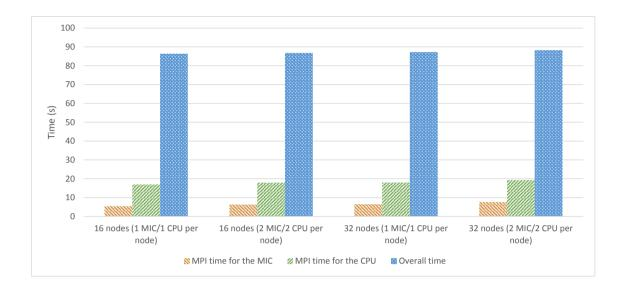
Figure 5.87: Performance of section S3 of algorithms version 2 and version 3. The orange bar shows the maximum MPI time among the MICs' processe; the green bar shows the maximum MPI time among the CPUs' processes; and the blue bar shows the overall run time in seconds.
