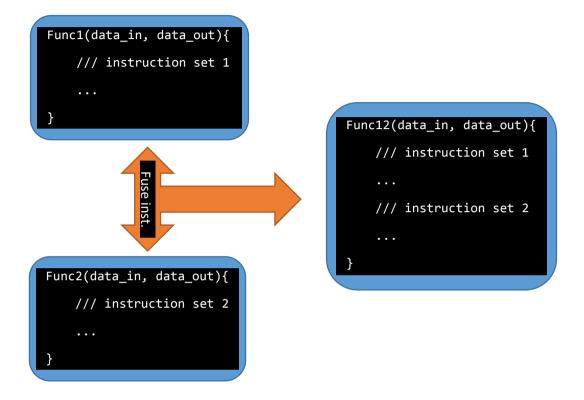
Figure 4.23: Fusing different functions that work on the same data. The instructions of the two functions on the left, in which the same set of data is processed within them, can be fused together to form the fused function on the right side.
