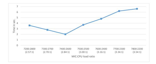
Figure 5.58: XFLAT timing benchmark on single-node (dual-CPU and dual-MIC) heterogeneous environment. The maximum time spent on MPI functions either CPU or MIC is shown for different MIC:CPU load ratios and runs employing 10k theta beams. Each point represents [number\_of\_theta\_angles\_on\_MIC : number\_of\_theta\_angles\_on\_CPU] (the normalized load ratio is shown in parenthesis).
