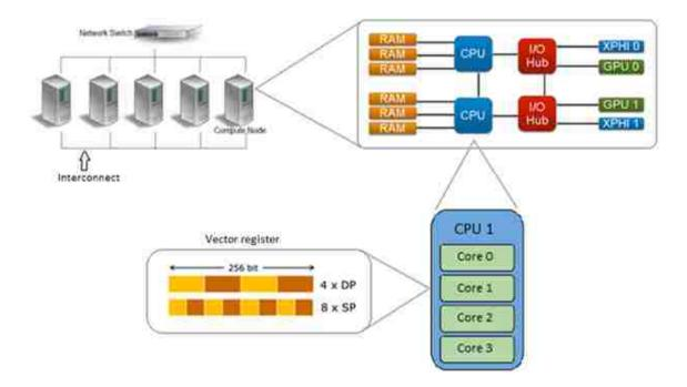
Figure 1.4: Cluster nodes and internal architecture of each node on a heterogeneous supercomputer. At the highest level compute nodes are interconnected via high-speed interconnect links. Inside each node, there may be multiple CPUs as well as accelerator cards. Typically, inside each processor there are a few to many cores. Finally, within each core, a vector instruction can be issued on multiple data simultaneously.
