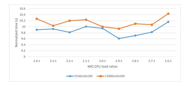
Figure 5.64: Stampede single-node benchmark for two different neutrino beam configurations,  $5550 \times 10 \times 100$  and  $12000 \times 10 \times 100$ , for various MIC:CPU load ratios. In order to compare the two curves on the same scale, the timings for them were scaled (normalized) (actual times in Table 5.18 and Table 5.19).
