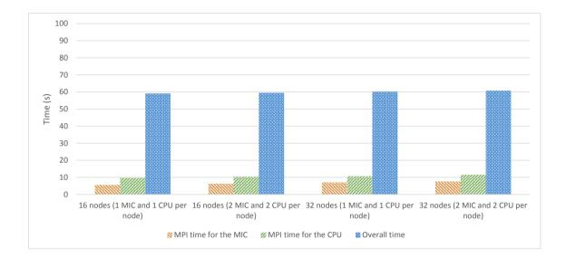
Figure 5.88: Performance of the last section before the last reduction for all algorithms. The orange bar shows the maximum MPI time among the MICs' processes; the green bar shows the maximum MPI time among the CPUs' processes; and the blue bar shows the overall run time in seconds.
