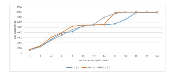
Figure 5.97: XFLAT performance over a range of compute nodes. The problem size was  $10000 \times 10 \times 100$ . The run time was continued for 100 seconds and the number of computed radial steps was measured. The blue curve shows XFLAT performance when the MIC:CPU ratio is 4; the orange curve shows XFLAT performance when the MIC:CPU ratio is 3; and the grey curve shows XFLAT performance when the MIC:CPU ratio is 2.
