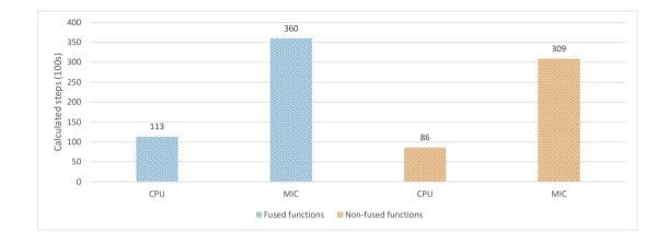
Figure 5.28: Performance of fused and non-fused functions on the CPU and the MIC on Stampede. The net computed radial steps (listed at the top of the bars) were measured for  $\sim 100$  second runs. XFLAT performance was 15% and 30% higher on the MIC and CPU, respectively, when the fused functions were employed (blue bars), compared to when the non-fused functions were employed (orange bars).
