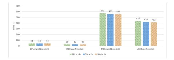
Figure 5.18: Performance of the CPU and MIC in two scenarios (implicit and explicit) on Stampede for different loop lengths (outer\_loop\_len × inner\_loop\_len). The kernel was benchmarked for three different loop combinations (scenarios):  $1M \times 10k$  (green bars),  $5M \times 2k$  (blue bars), and  $10M \times 1k$  (orange bars).
