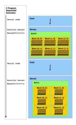
Figure 2.6: Launch of kernels from host. Host and device can have their own executions (shown in blue). Multiple grids (shown in green) can be launched from the host (Figure from NVIDIA 2014).
