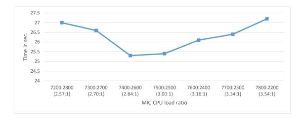
Figure 5.52: XFLAT timing benchmark on a single-node heterogeneous environment. Execution time shown for different MIC:CPU load ratios using 10k zenith trajectories. Each point represents [number\_of\_theta\_angles\_on\_MIC : number\_of\_theta\_angles\_on\_CPU] (the normalized load ratio is shown in parenthesis).
