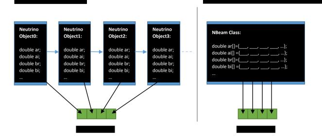
Figure 4.17: XFLAT data access pattern for AoS and SoA approaches. In the AoS approach (shown on the left), in order to fill up a SIMD register (shown in green), fragmented data must be extracted from multiple objects (shown in blue). On the other hand, in the SoA approach (shown on the right), multiple data can be loaded simultaneously into a register with a single continuous fetch.
