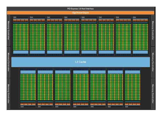
Figure 2.3: Full chip block diagram of NVIDIA GK110 architecture containing clusters (Streaming Multiprocessors) of CUDA cores. Blocks can share data using the shared L2 cache unit (shown in light blue in the middle), and each one can access the global memory outside the chip through memory controllers (shown in grey on the sides) (Figure from NVIDIA 2012).
