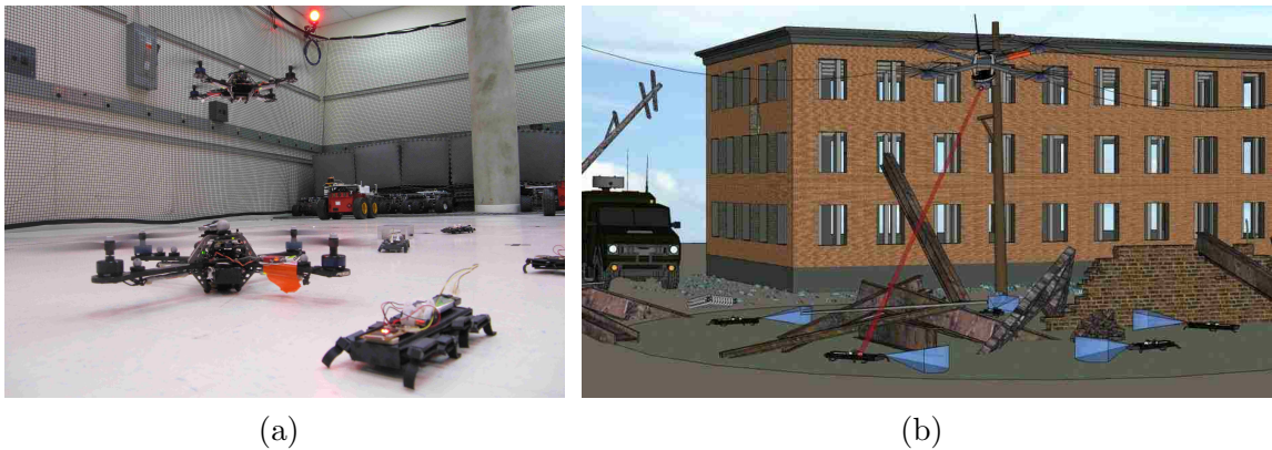
Figure 1.1: (a) A group of OctoRoACH crawling robots together with a group of quadrotors. (b) Mission scenario: a quadrotor used as communication relay for a team of ground mobile sensors that are deployed to explore a disaster area. This sketch also shows an optical wireless communication link between the quadrotor and one of the mobile sensors.
