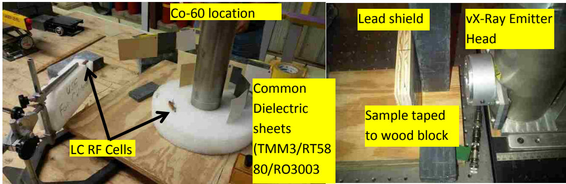
Figure 49 Pictures of Cobalt (left) and X-Ray (right) setup for the exposures on the samples.
