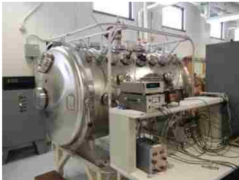
Figure 57 Custom built Jumbo chamber for simulated space exposure
