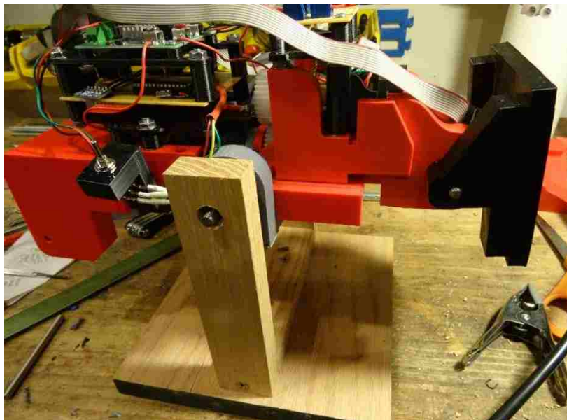
Figure 74. Experimental apparatus for determining link mass properties
