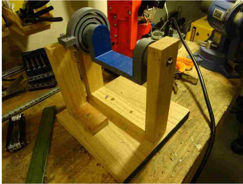
Figure 74. Experimental apparatus for determining link mass properties
