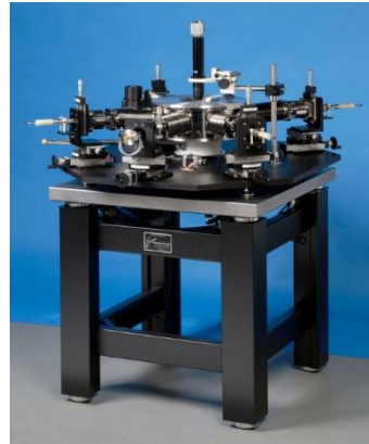
Figure 17: Example of a Micro-manipulated Probe Station Research Test Setup from Janis Research Co. [26]
