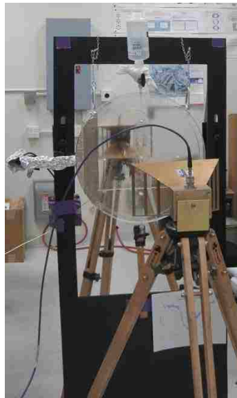
Figure C.3. Frequency calibration setup for the microwave calorimeter.
