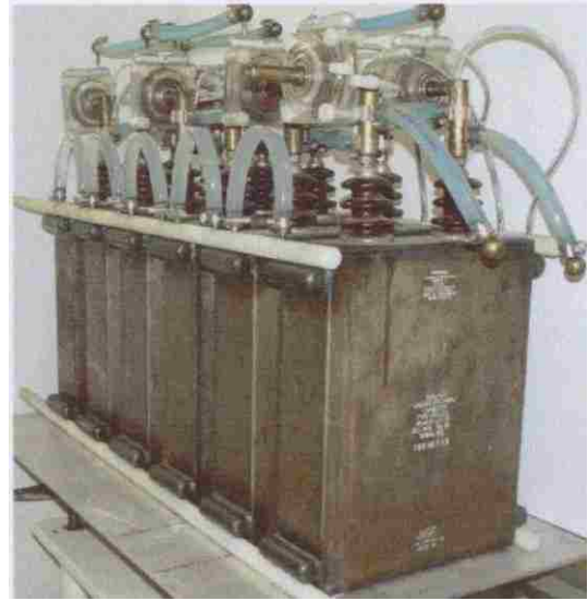
Figure 4.3 An equivalent circuit diagram of the Marx bank (left), and a photograph of the Marx bank being maintained before installation in the accelerator (right).
