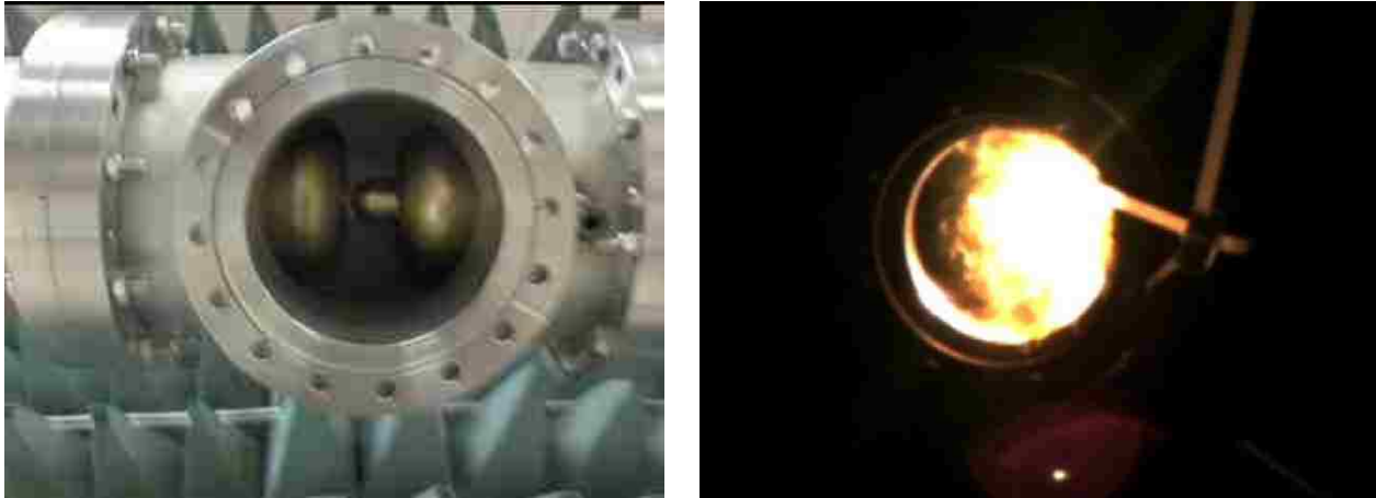
Figure 4.5 Photographs of the 2 ns self-break oil switch during switch characterization. Looking through the view port before firing (left), and during firing (right).
