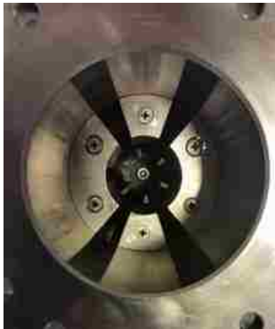
Figure 1.4 The view from the extraction port of the A6 magnetron, with the simple mode converter installed.
