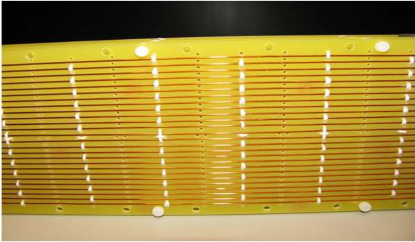
Figure 5.3 Winding structure turns and their isolation.
