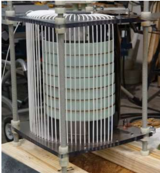
Figure 5.5 Photograph of the final build of the pulsed primary switch.
