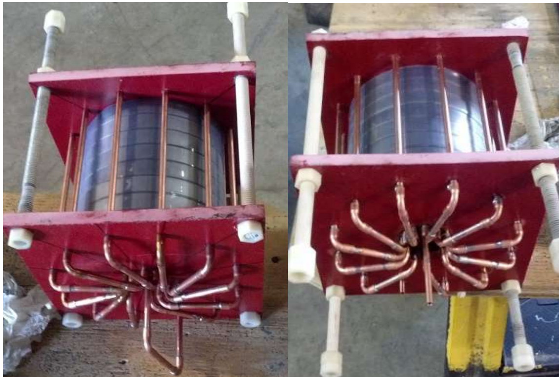
Figure 5.4 Photograph of the 12-turn MnZn saturating switch.
