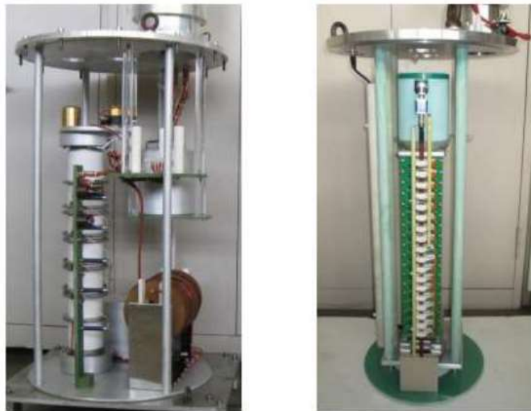
Figure 1.2 Solid replacement for a thyatron switch [6].
