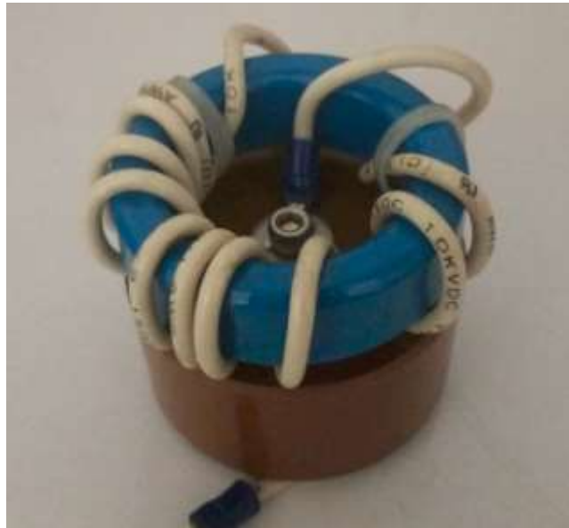
Figure 5.6 Photograph of the magnetic delay circuit out before installation.
