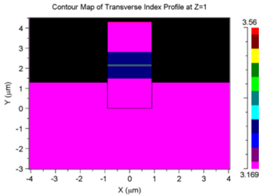
Fig. 5.1. Transverse refractive index profile of InGaAsP/InP QW ridge waveguide laser
