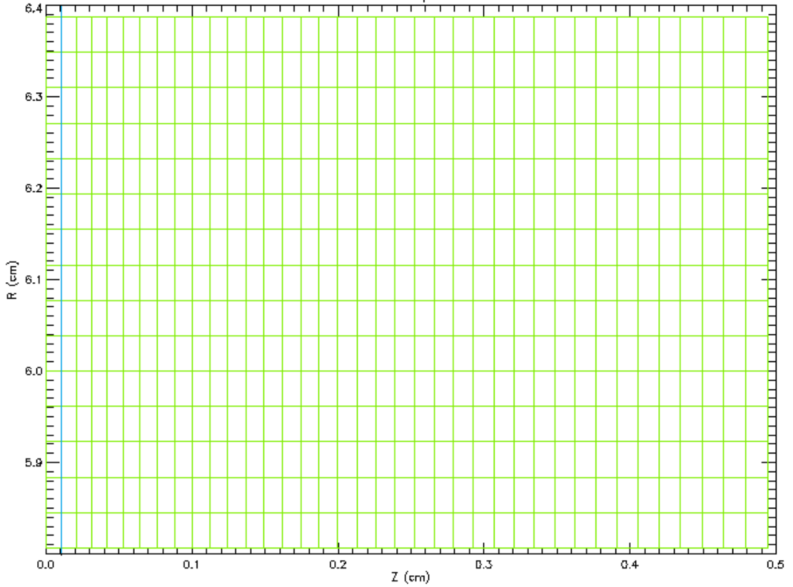
Figure 2.2: An example of the nonuniform gridding near the anode foil (blue line on left) in the PRD simulation. The smallest dimension is 0.0101 cm and the largest dimension is 0.0399 cm.
