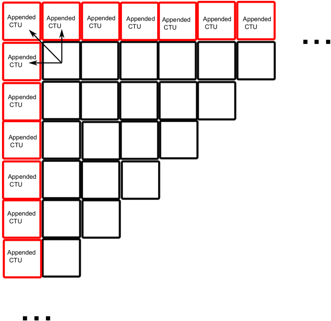
Figure 4.4: Model updates for the first row and column. The virtual CTU encodings assume the Pareto front that is initialized from other videos and then updated based on the encodings of the first few frames of the current video.
