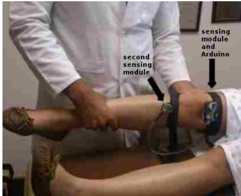
Figure 2.17: The pivot shift tester, one sensing module located in the tibia and the second one in the femur
