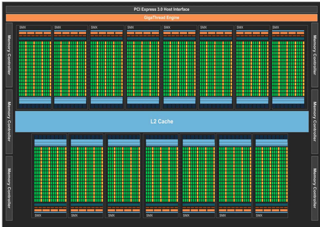
Figure 2.3: Kepler Block Diagram
