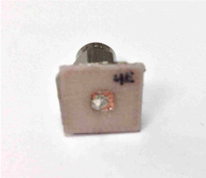
Figure 3-20: 25 Ghz Antenna Made With Copper Tape And Conductive Epoxy
