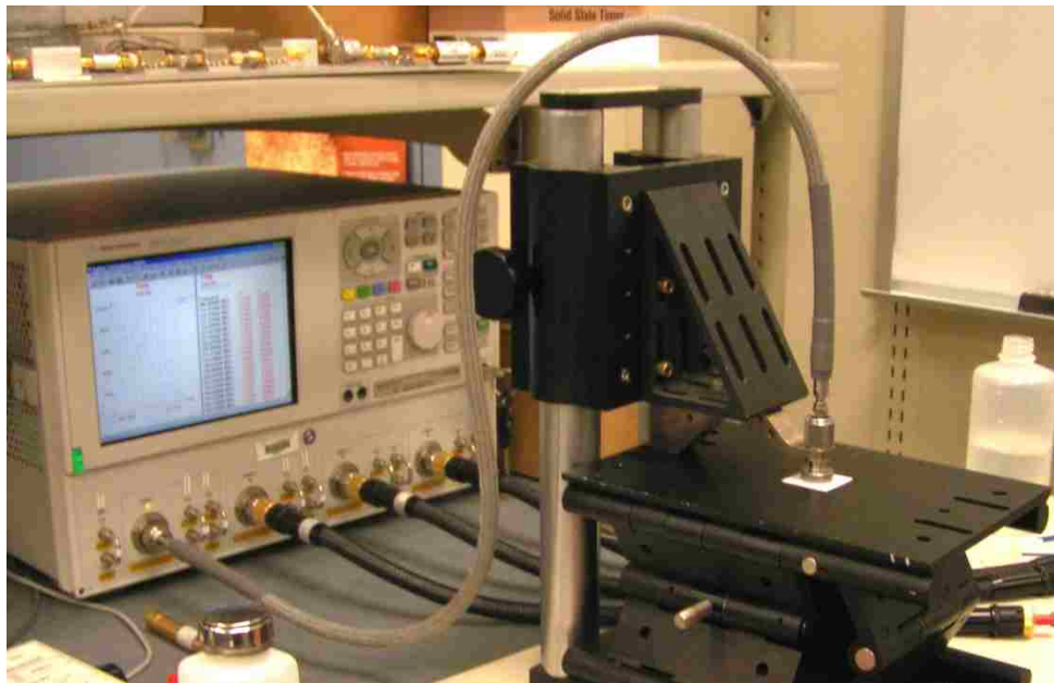
Figure 2-5: Dielectric Probe Set-Up
