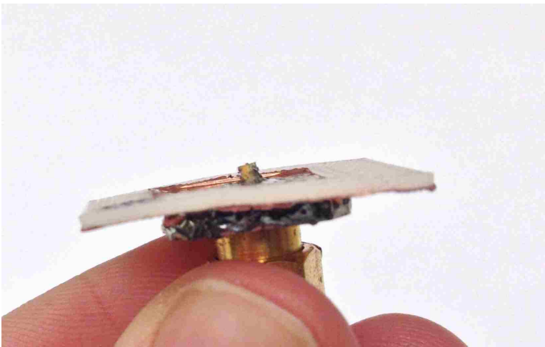
Figure 3-17: 10 GHz Antenna Warped From Soldering Heat
