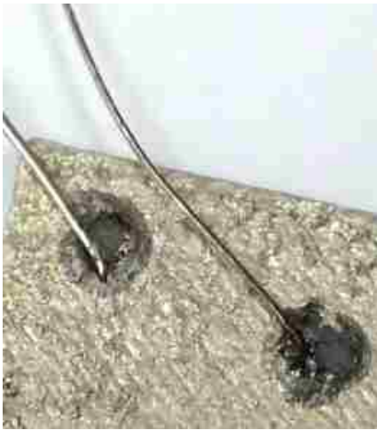
Figure 3-14: Conductive Paint Melting Away From Solder
