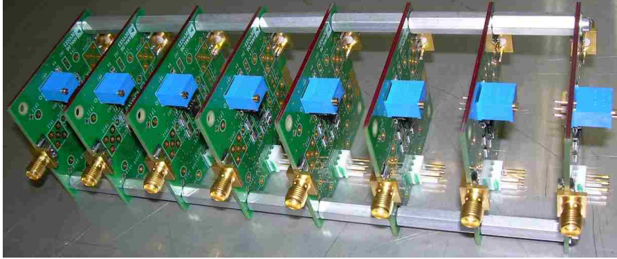
Figure 2.9: A set of 8 amplifiers to amplify the I and Q signals of four interferometer chords. Two such sets were built. The SMA terminals which are centered (near the camera) are the outputs and the offset SMA terminals are in the inputs (far from the camera).
