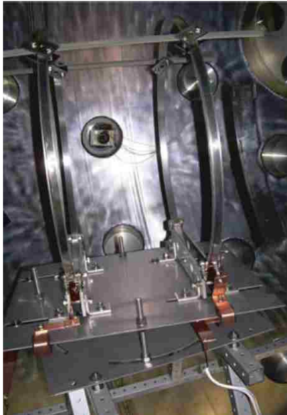
Figure 2.3: View of the in-vacuum Helmholtz coils, with end-on view of far railgun bore visible. Copper buswork, prior to insulation attempts, is visible in the bottom of the image. Image from [25].
