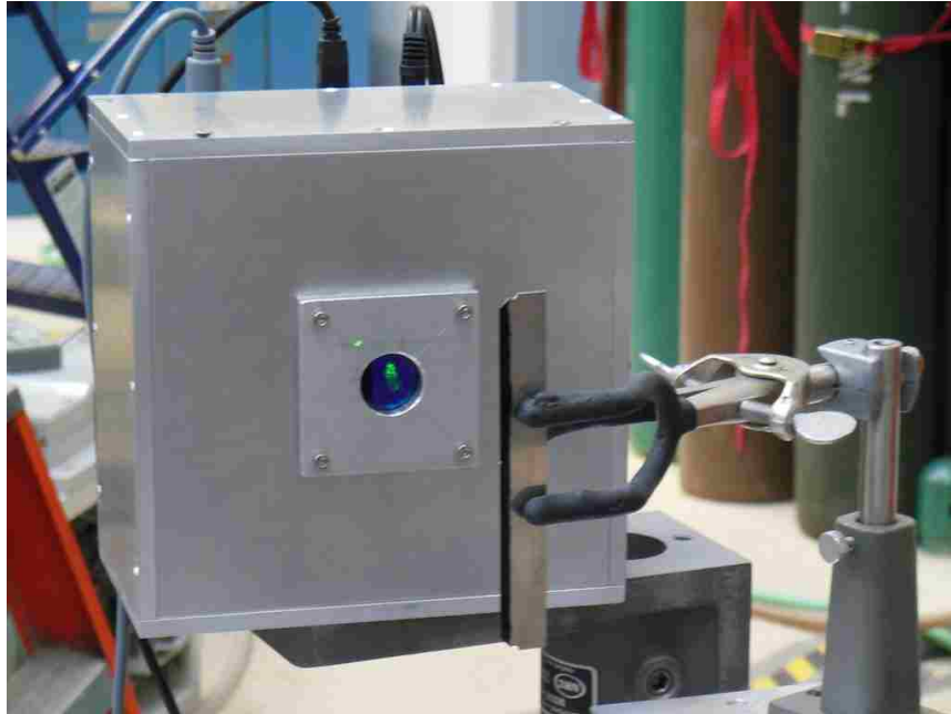
Figure 3.4: The Apogee imaging unit is located on the back of the aluminum enclosure containing two filters. The knife edge mount is translatable transverse to, and along the beam at the focal point of the second parabolic mirror. The green (532 nm) alignment beam is incident on the knife edge and filter.
