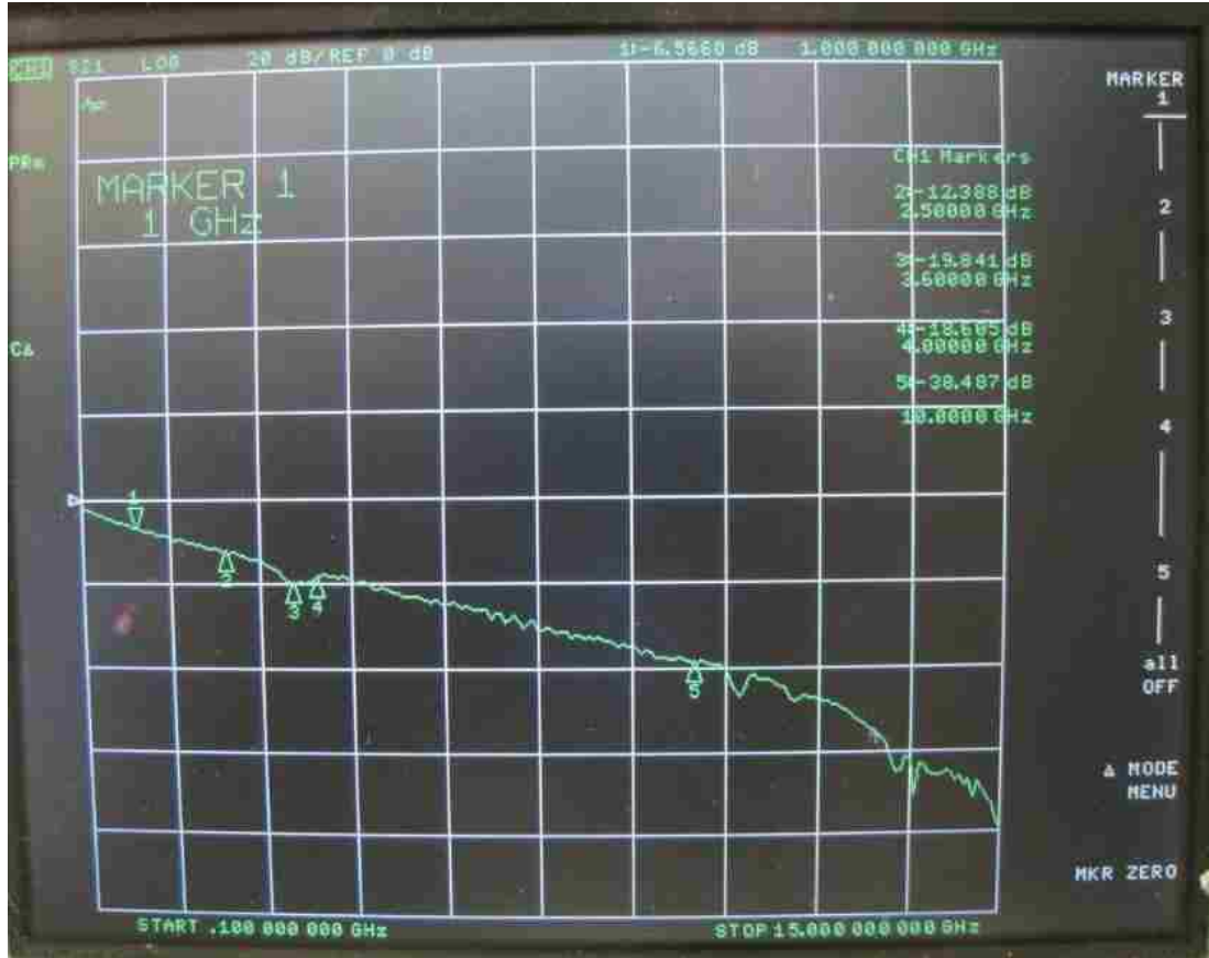
Figure A10. "Purple" cable set RG-214 attenuation vs. frequency.
