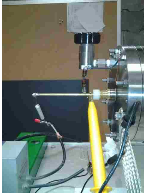
Figure 4.2.1. D-dot probe calibration setup.
