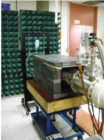
Figure 4.2.6. Calorimeter in use for a UNM BWO experiment that outputs a simultaneous TE_{11} and TM_{01} mode.
