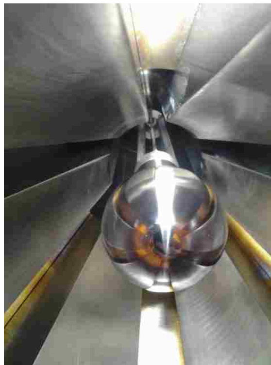
Figure 3.2.8. Photograph of the polished stainless-steel spherical endcap used in MDO experiments that was based on the MAGIC designs.
