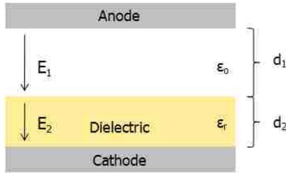
Figure 2.1.10. The electric field strength on the cathode surface is 1/\epsilon_r of that with no dielectric coating.
