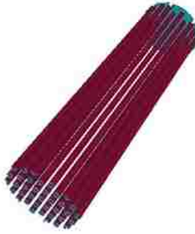
Figure 3.2.49. Schematic of a rodded cathode.
