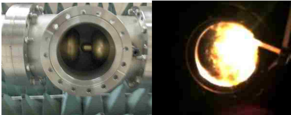
Figure 4.1.2. Low-inductance 2-4 ns oil breakdown switch.
