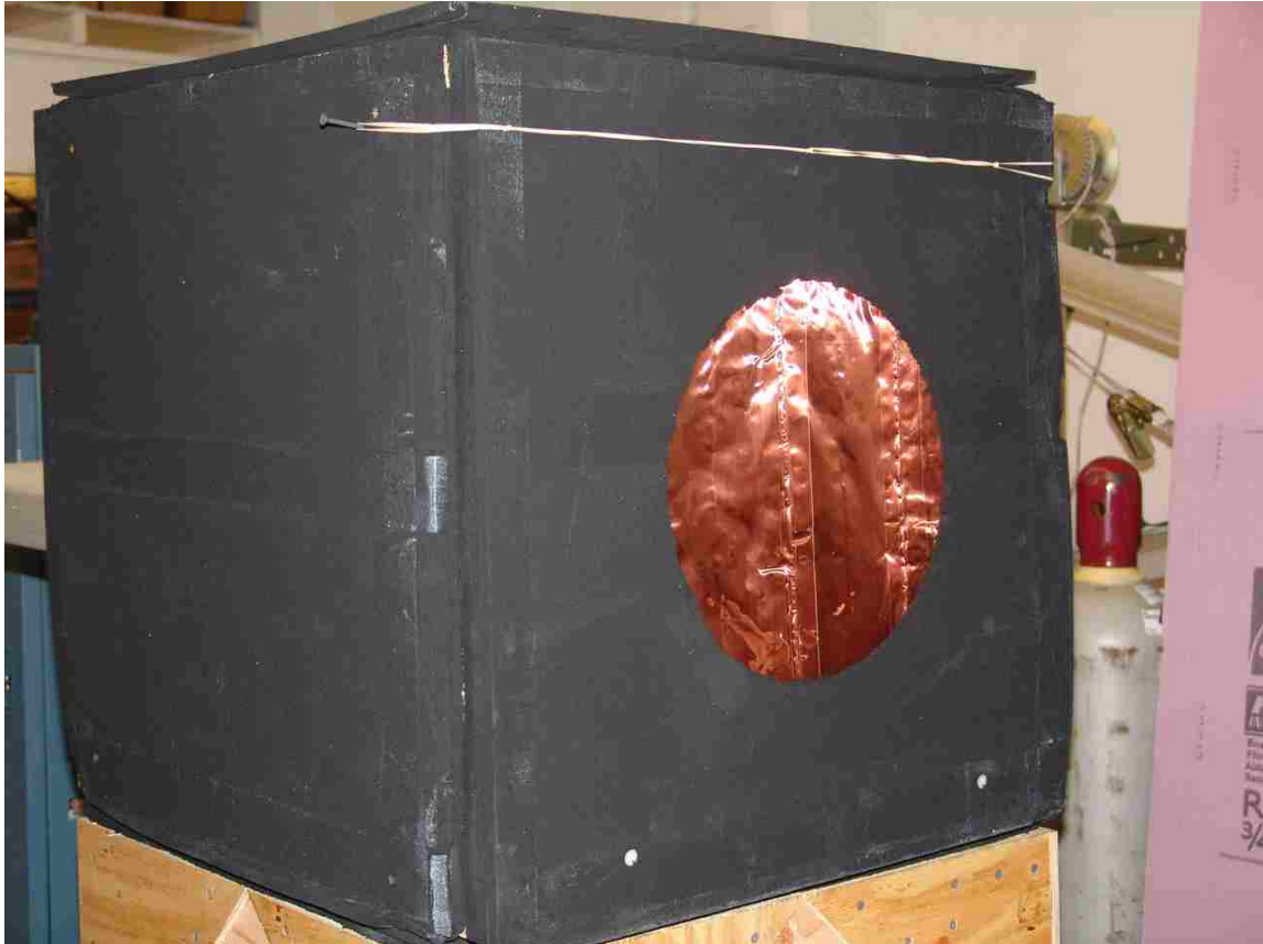
Figure 80. Absorber Box with Copper Sample for Impulse Tests
