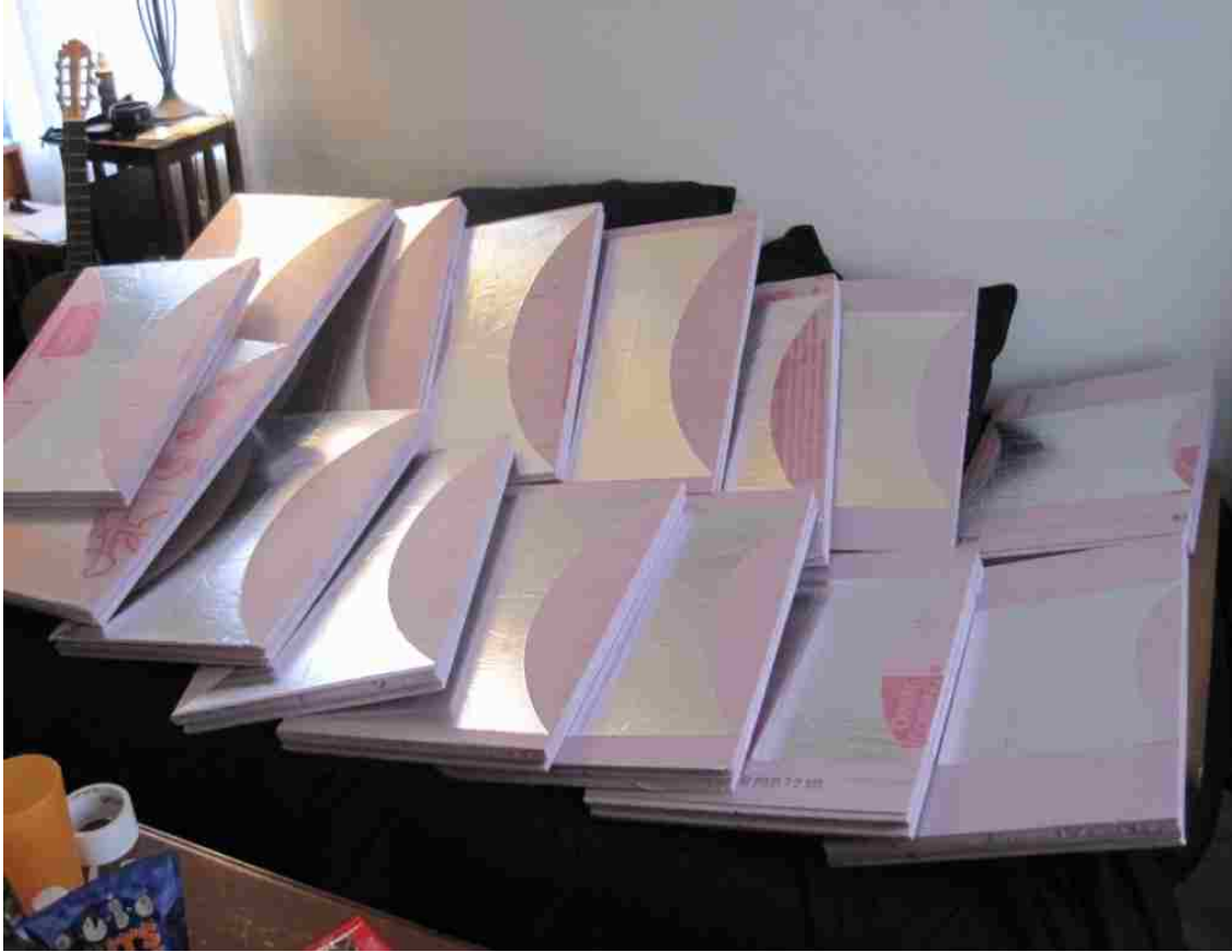
Figure 11. 5GHz prototype lens plates prior to assembly
