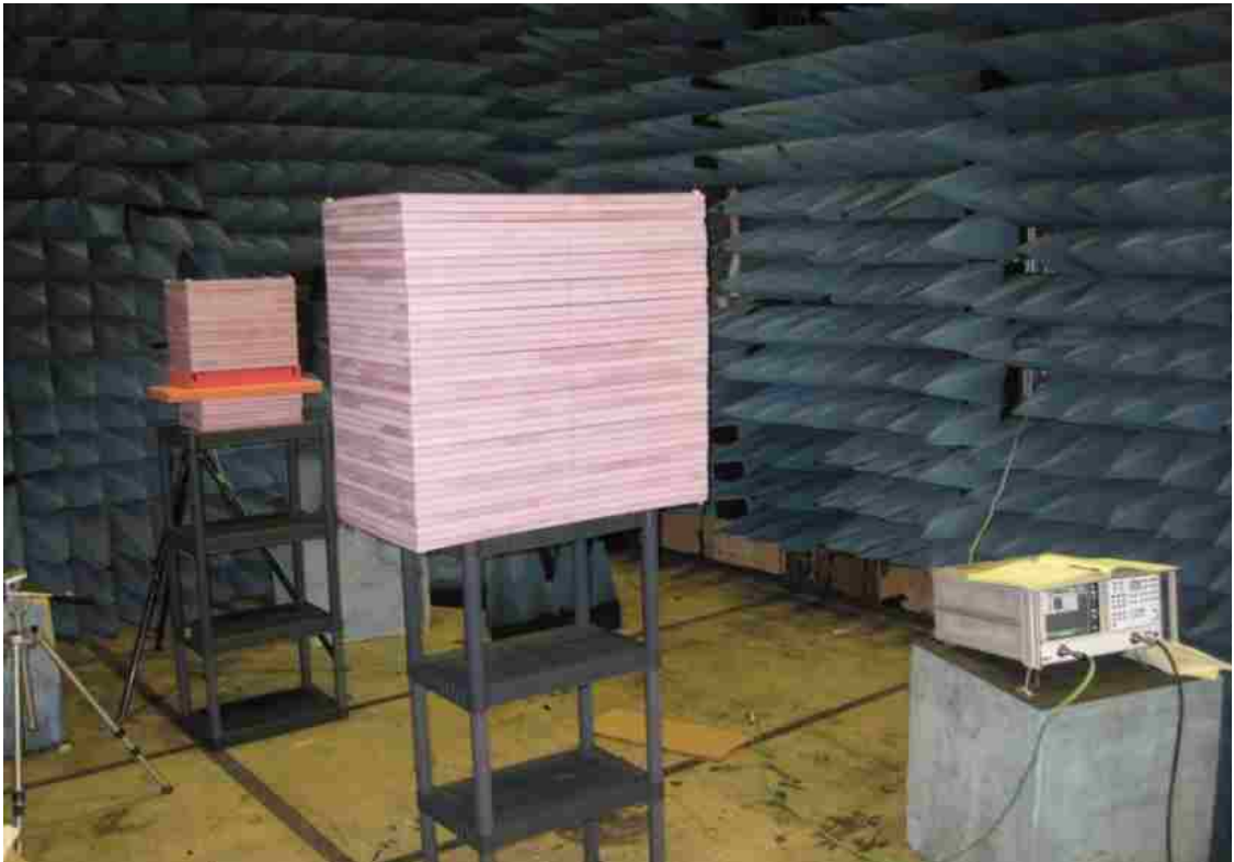
Figure 60. Test Setup; Lenses Positioned for Beam Collimation
