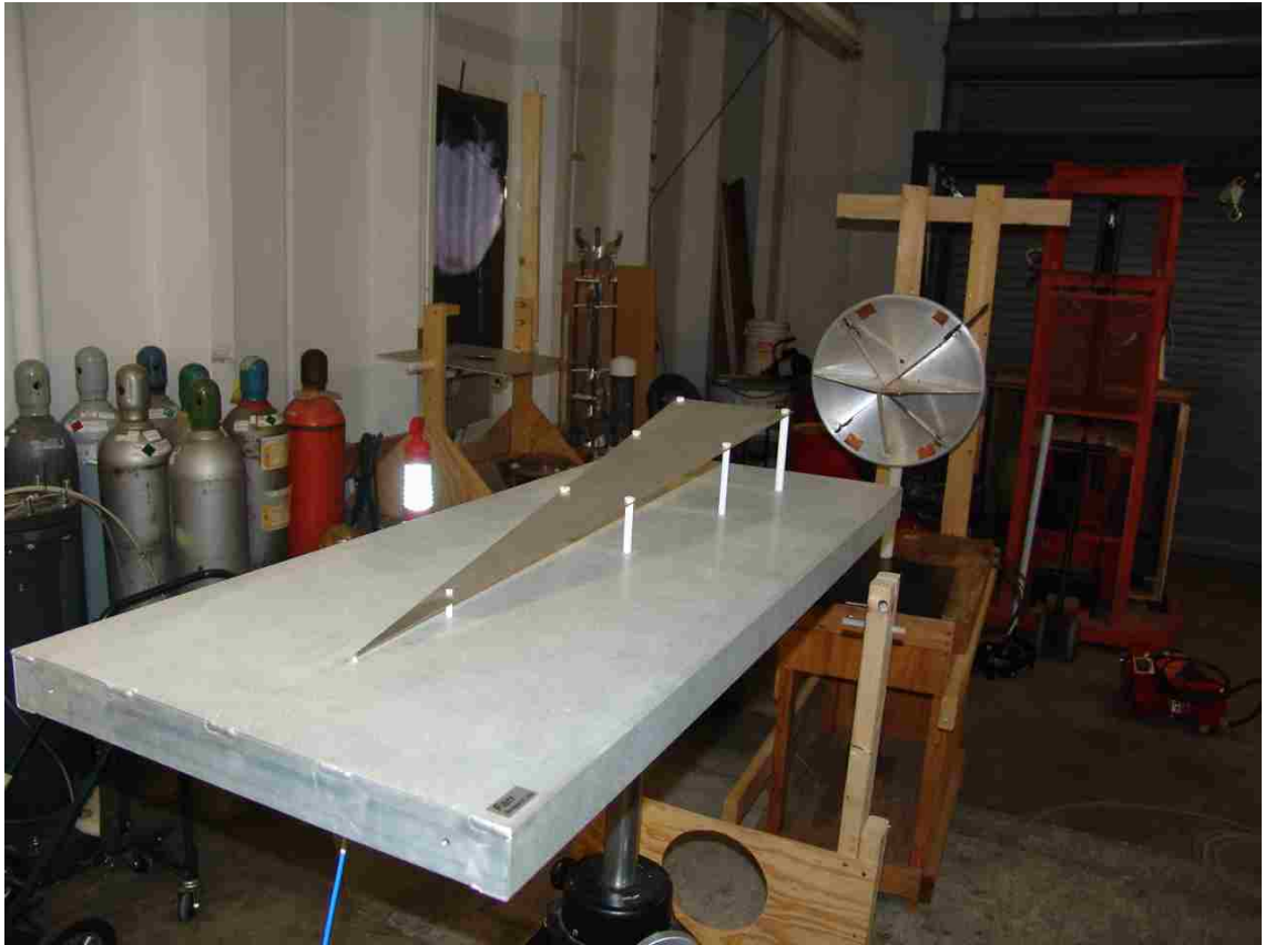
Figure 77. Transmit and Receive Antennae Used in Impulse Tests
