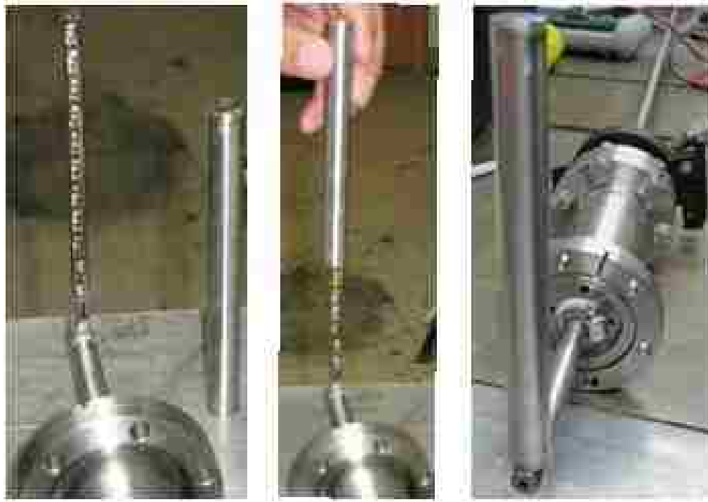
Figure 2.31. Stainless steel tube installation to eliminate electrostatic pick up.
