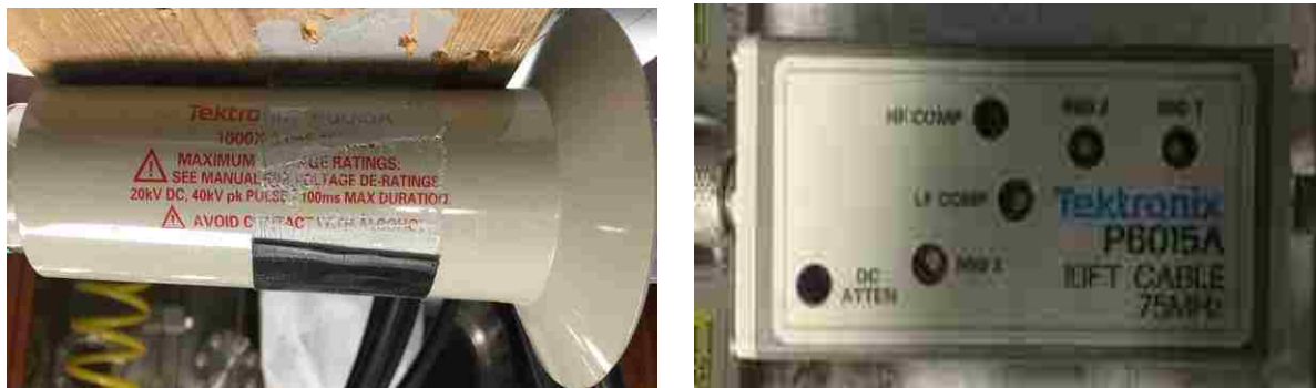
Figure 2.22. High-voltage probe P6015A for discharge voltage measurements.
