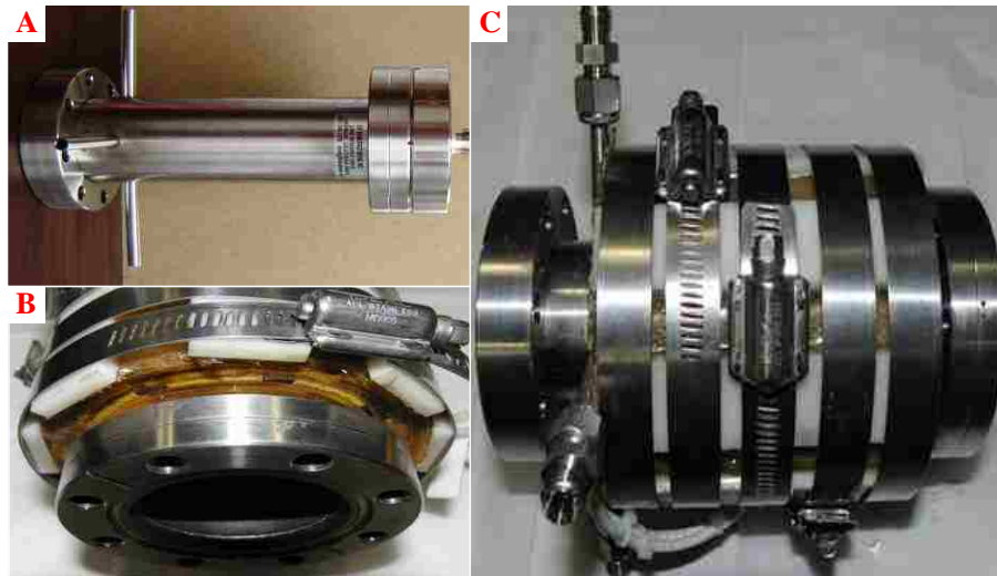
Figure 2.9. A: Picture of the cylindrical body of the plasma gun before adding the solenoidal bias coil; B: Partial side-view picture of the gun after bias coil installation; C: Top-view picture of the gun after the bias coil is installed.
