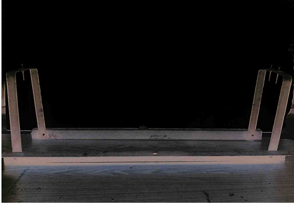
Figure 37: LVDT reference frame for 229 mm (9 in) deep specimens
