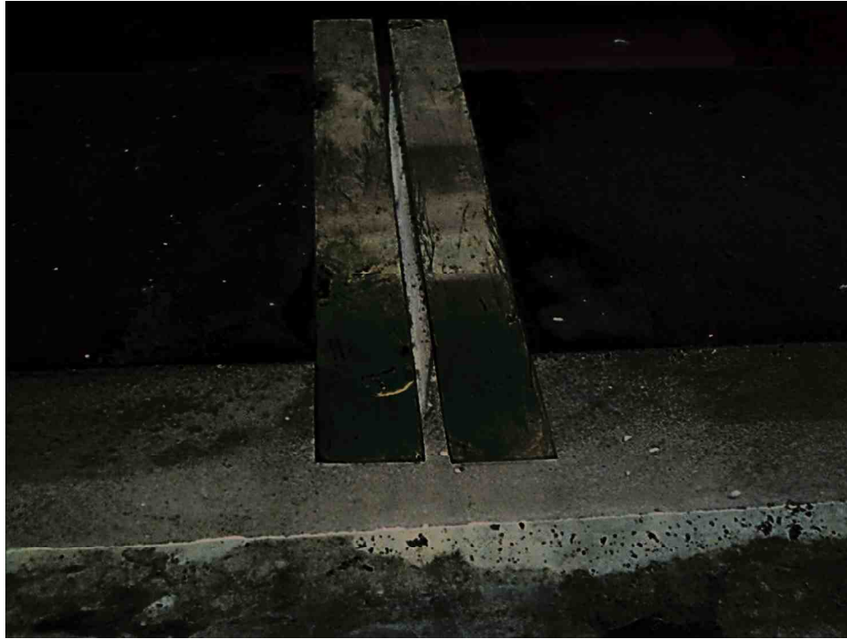
Figure 40: Photograph of beam after gluing knife edges
