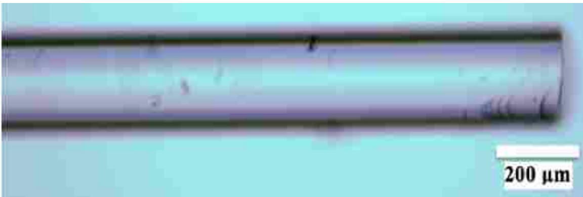
Figure 5.8: Micrograph of a ZBLAN fiber processed at 300°C for 60 seconds.
