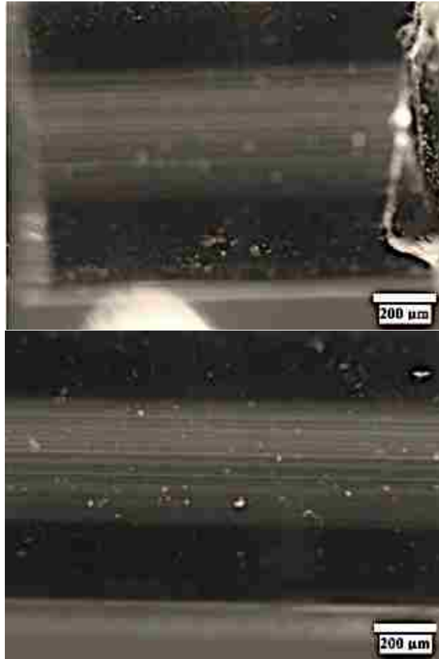
Figure 4.31: Polarized micrograph of ZBLAN sample processed at 290°C in hyper-g (top) and 1-g (bottom).
