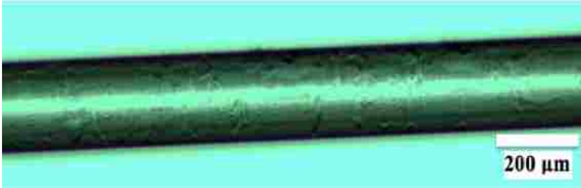
Figure 5.12: Micrograph of a ZBLAN fiber processed at 360°C for 8 minutes.
