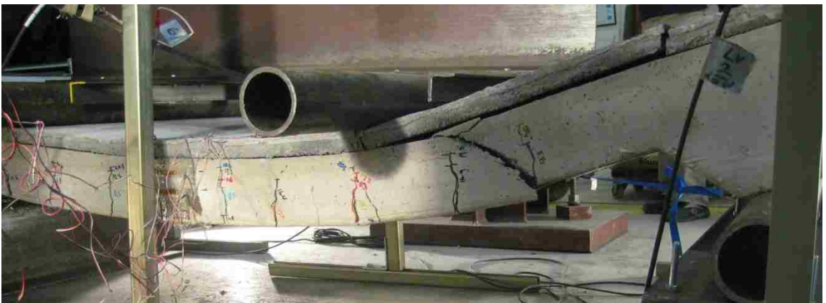
Figure 5.24: Shear failure in the NVC
