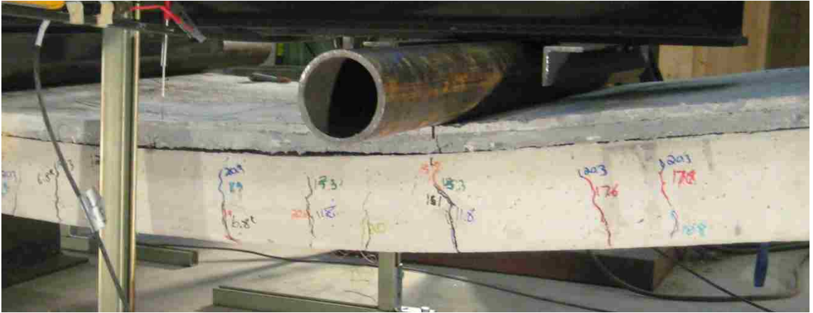
Figure 5.23: UHPC and NVC slab after buckling
