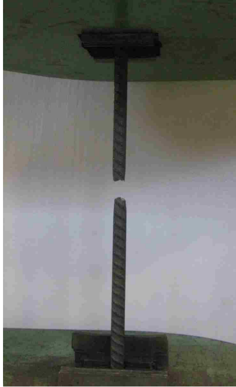
Figure 3.30: Direct tension test of the flexural steel
