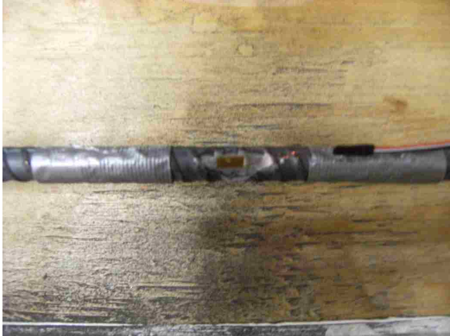
Figure 3.16: Strain gauge on a reinforcement bar
