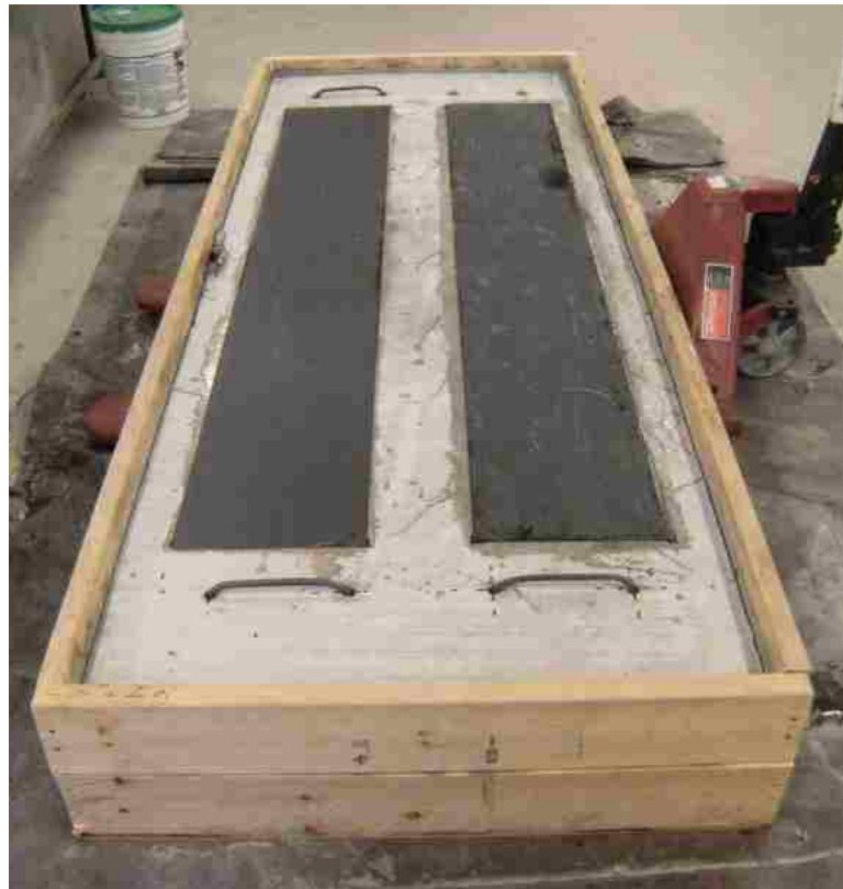
Figure 3.23: CFRP and shear-friction reinforcement
