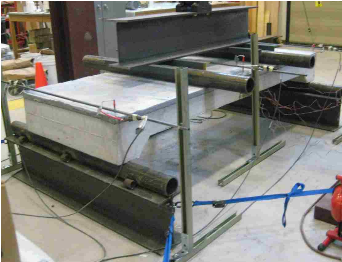
Figure 3.34: The strengthened slab prior to testing
