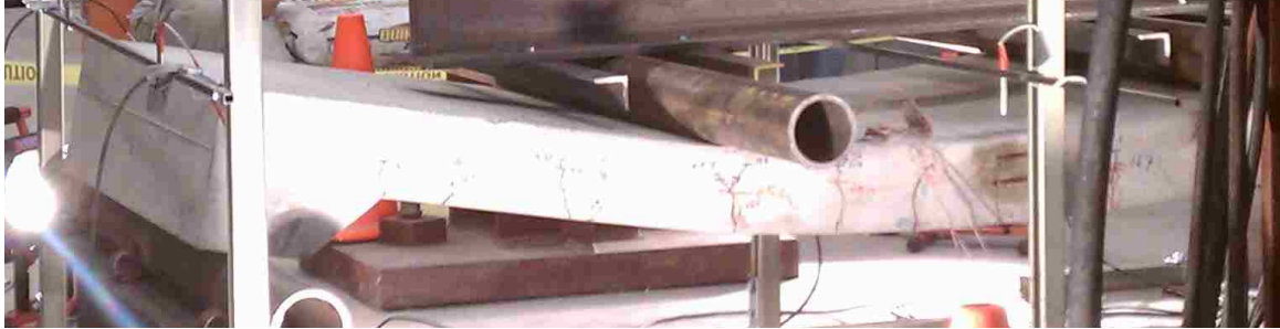
Figure 5.2: Deflection of the control slab near failure
