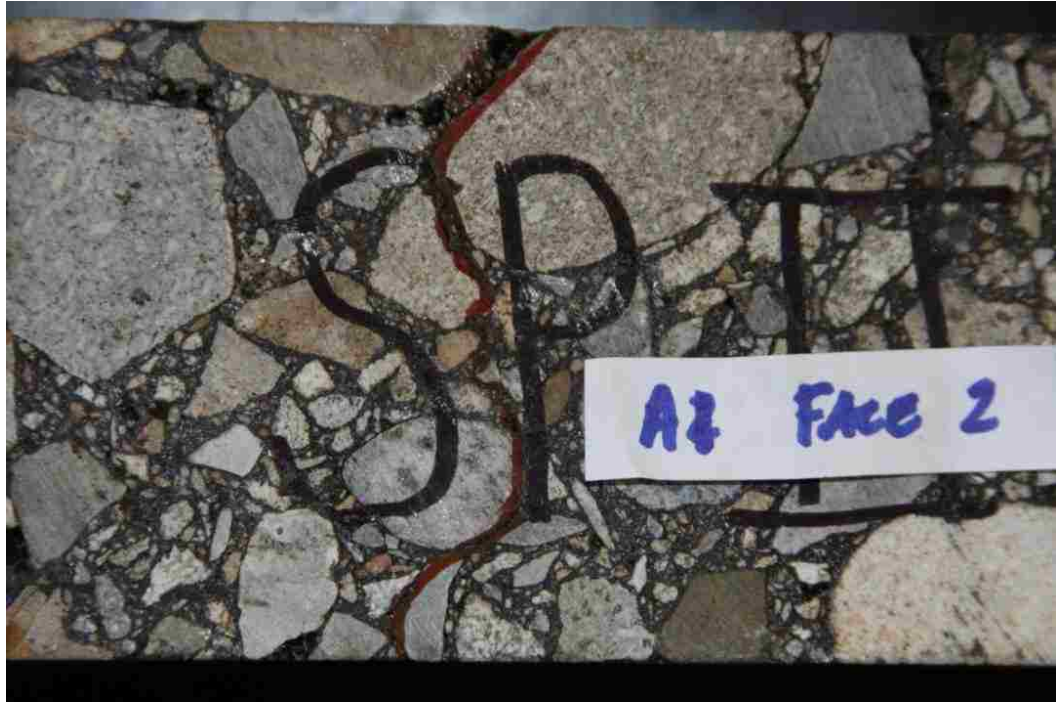
Figure 6.1 Fatigue Cracking in HMA Beam Sample SP-II-A1
