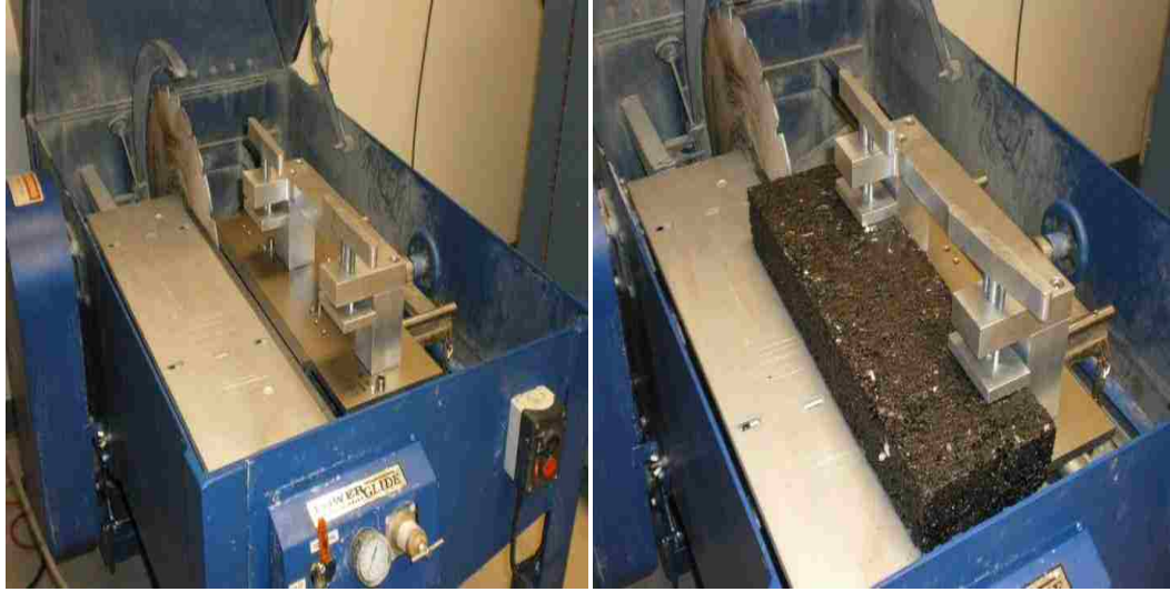
Figure 3.6 Stone Cutting Saw with Modified Clamp
