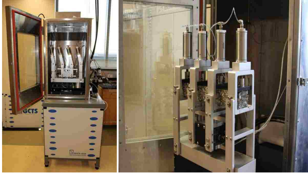
Figure 3.7 Environmental Chamber and Beam Fatigue Apparatus
