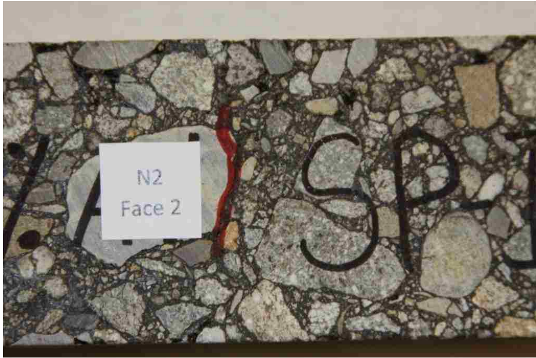
Figure 6.4 Fatigue Cracking in HMA Beam Sample SP-II-N2
